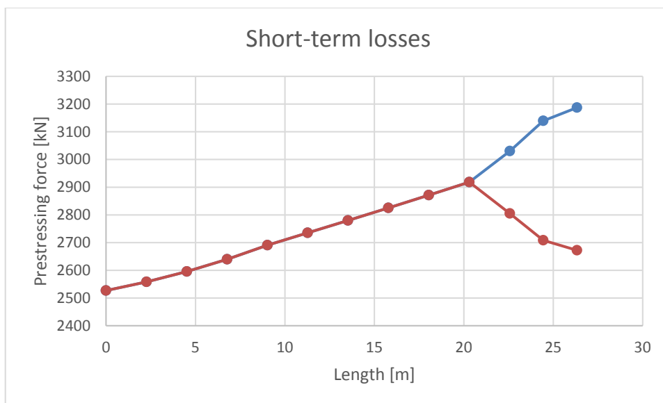
Figure 26 Short-term losses for the cable from the 1 st stage.
