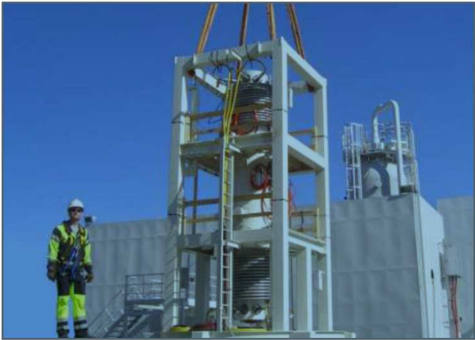
Figure 3.4 Gullfaks: Wet gas compressor prototype WGC4000 (Hjelmeland, Olsen et al., 2011)
