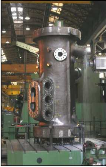
Figure 3.3 Ormen Lange: Integrated motor compressor casing (Skofteland, Hilditch et al., 2009)
