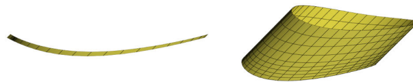
Figure 3.10: Left: first layer of elements, made of deformed ellipses. Right: Start of branch mesh.
