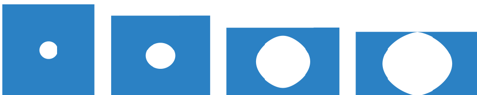
Figure 4.15: Deformation of the axisymmetric unit cell in generalized compression for triaxiality ratio \sigma^* = 2 .
