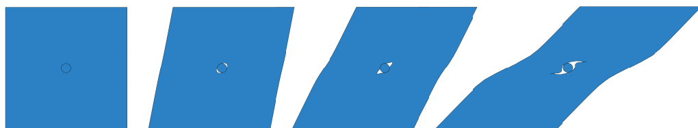
Figure 4.32: Deformation of the shear unit cell. Triaxiality ratio \sigma^* \simeq 0 .
