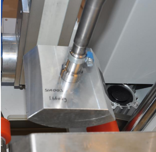
Figure 3-25: Impactor: Top view
