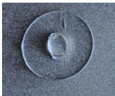
Figure 3-3: Imperfection at injection point
