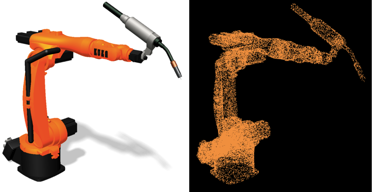
Figure 4.4: A CAD model of the KUKA KR5 robot and its resulting point cloud. The CAD model is here converted to 50 000 points.
