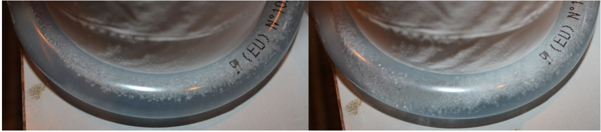
Figure 4.3: Flow regime in one loop coil. Left picture shows stable bubbly flow with smooth bubble distribution. Right picture shows unstable bubbly flow with irregular bubble distribution.
