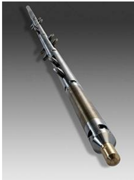
Figure 2.4: Illustration of well tractor without drill bit(AkerSolutions 2013).
