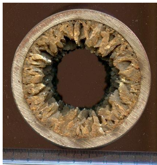
Figure 2.8: Scale build up in 3-inch pipe (BP 2010).
