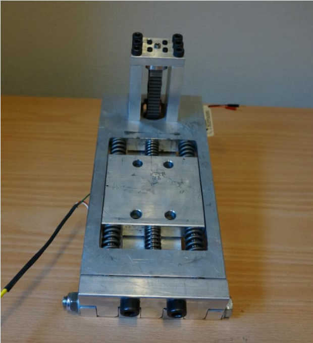
Figure 3.3: The rig showing sliding plate and springs.
