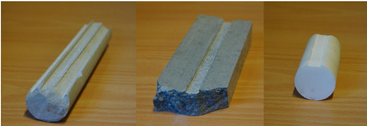
Figure 4.1: Stones used for testing, from the left: Berea Sandstone, Grunnes Soapstone and Dionysos Marble.
