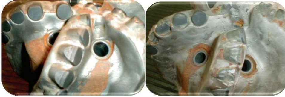
Figure 2.3: Bit wear without and with stick slip failure(Deen, Wedel, and Nayan 2011).
