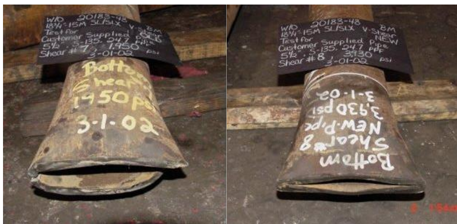
Figure 0.1 Shear test on old (left) and new (right) pipe (West Engineering Services Inc., 2002). Even though both pipes have the same specification, the new pipe required almost 2000 psi more to shear than the old pipe.
