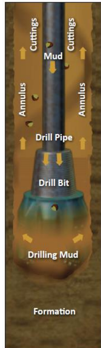
Figure 0.2 Drilling operation (National Commission on the BP Deepwater Horizon Oil Spill and Offshore Drilling, 2011)
