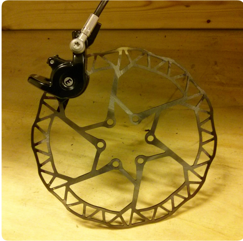
FIGURE E.1: engaging the caliper with disk
