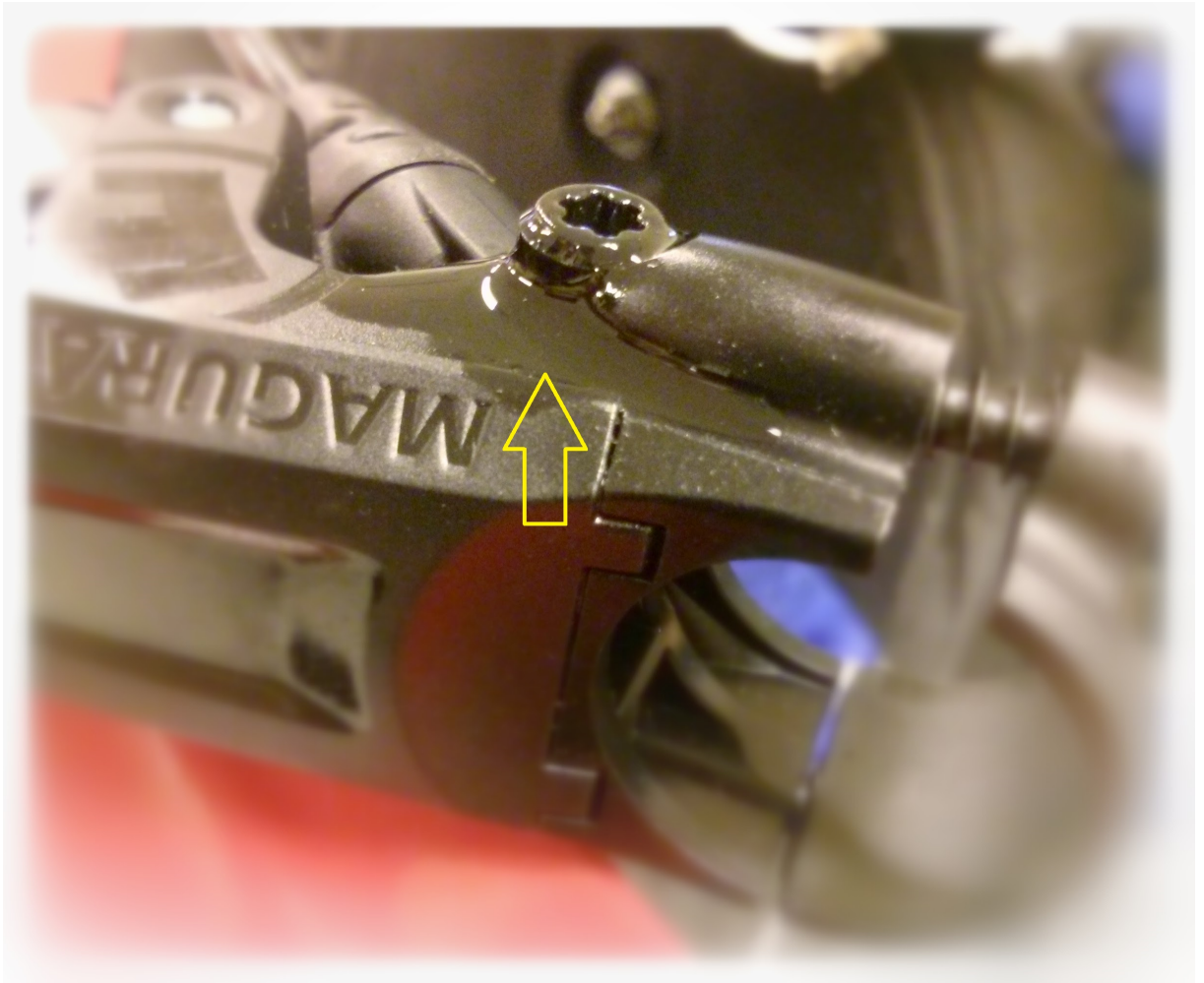
FIGURE E.4: Leakage around the lever bolt
