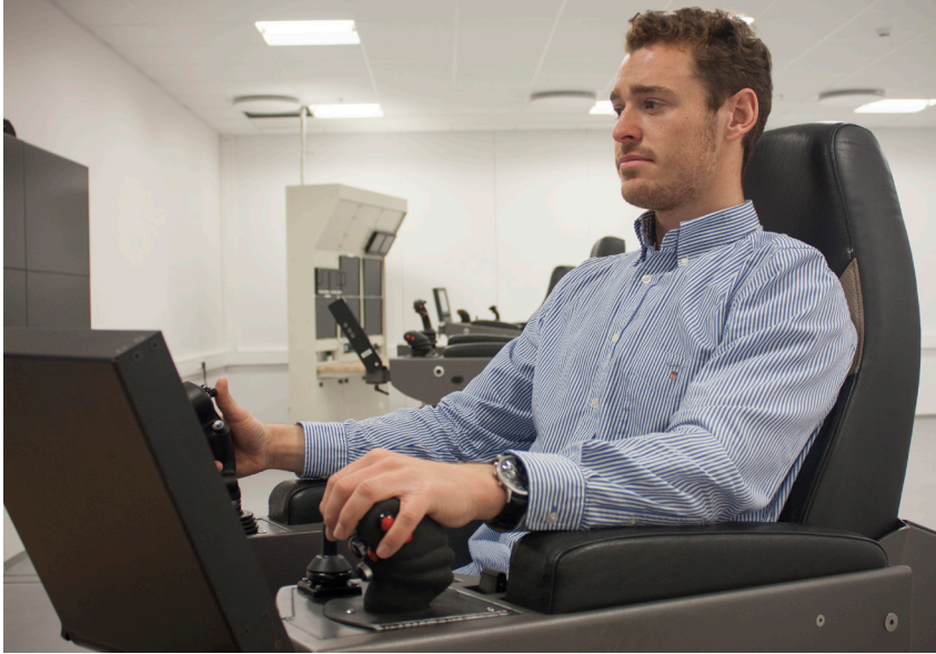
Photo 1: ROV Simulator used to train pilots at Oceaneering in Stavanger, Norway. The right joystick controls the ROV, while the left controls the simple manipulator.
