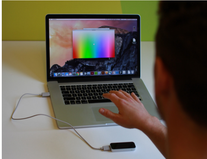
Photo 1: The Leap Motion test. The user moves his hand to move the colored background on the x-axis. A dot is added for positional reference.
