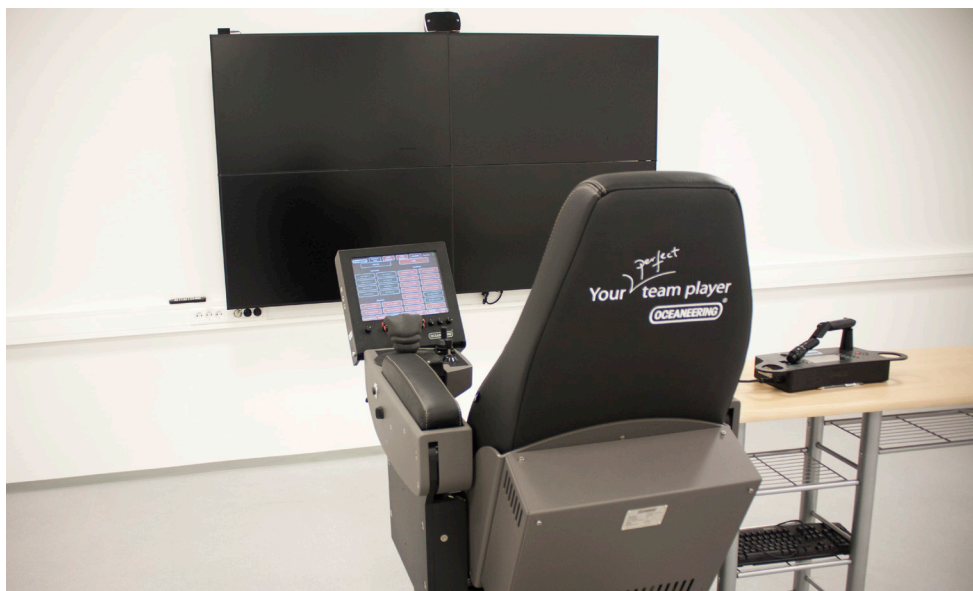
Photo 3: The most modern simulator gear at Oceaneering. To the right is the master arm that controls the advanced manipulator on the ROV.
