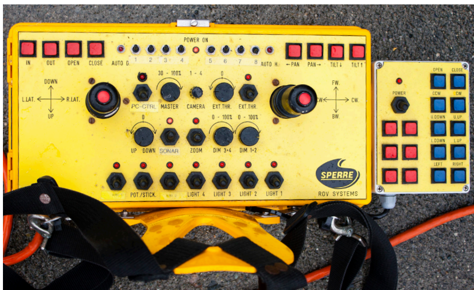
Photo 4: Portable controls for the Minerva ROV used by NTNU, using a double joystick setup.
