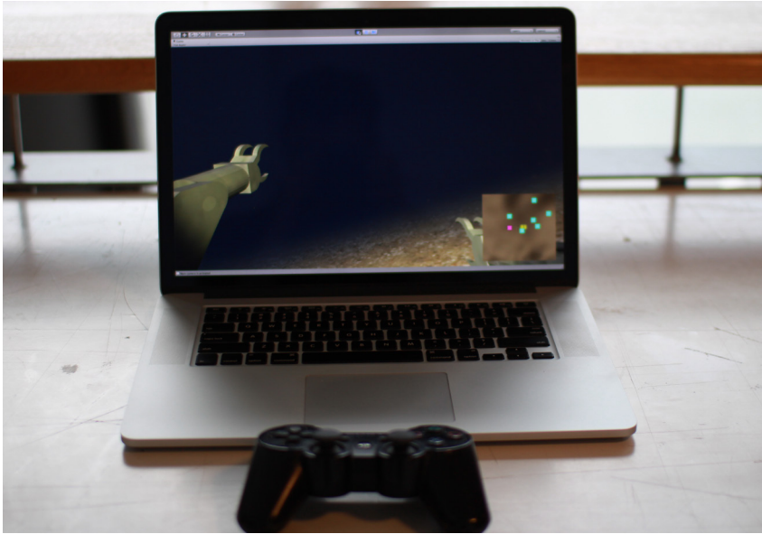
Photo 1: The Real condition. Visibility is bad, and the user has to navigate using the 2D map. The ROV is controlled by the PS3 controller.
