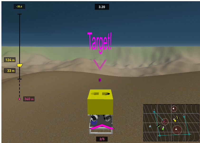
Screenshot 2: The user is in Follow mode, which is a 3rd person view of the ROV. It gives the user a better sense of the size of the ROV in relation to its surroundings.
