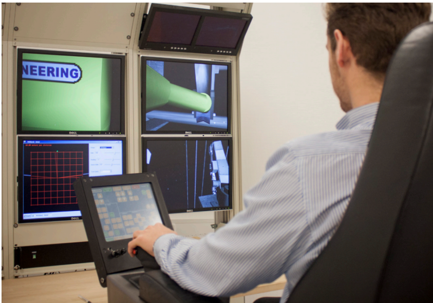
Photo 2: Screen layout for the Oceaneering ROV Simulator. Six screens display information to the pilot.
