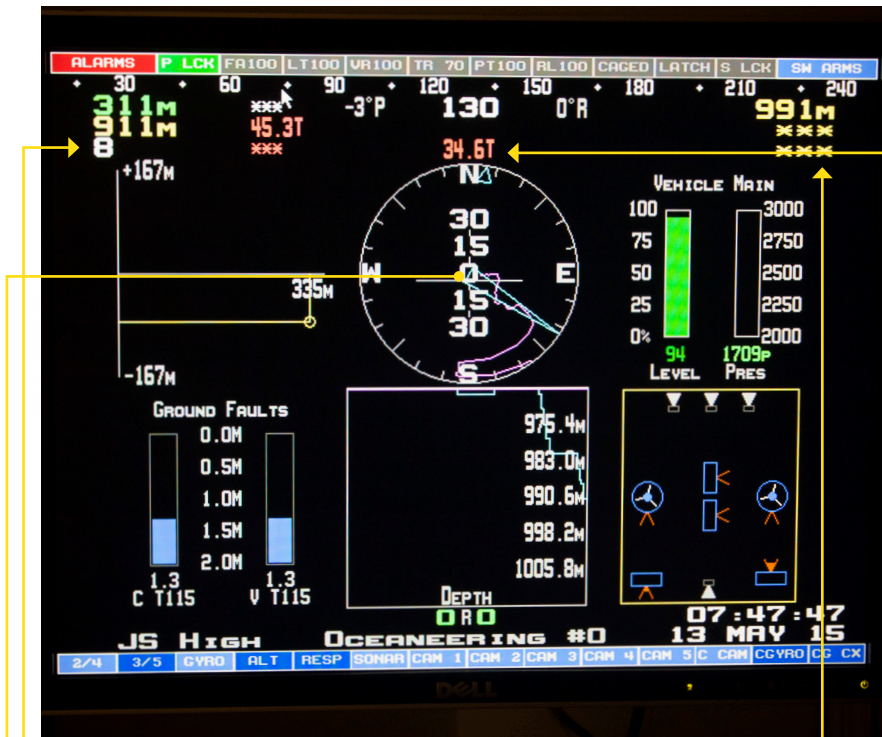
Photo 6 Display from the Oceaneering ROV Simulator showing direction, directional history, depth of ROV, depth of garage, altitude, netto rotations etc.
