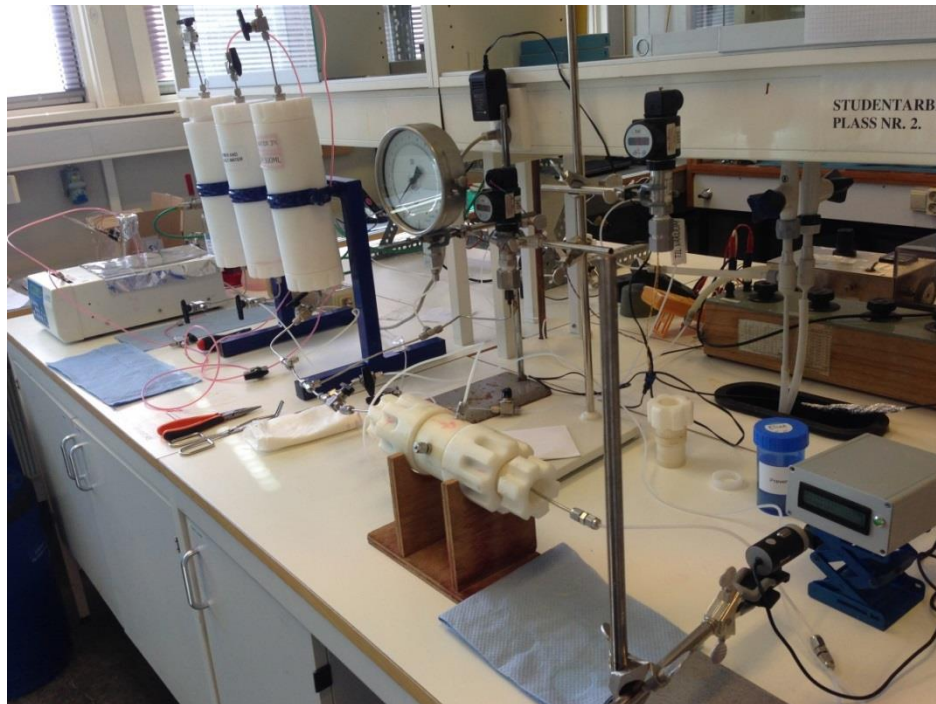
Figure 5.2 Experimental setup in lab. Showing pump, reservoirs, pressure transducer, core holder, and resistivity apparatus.
