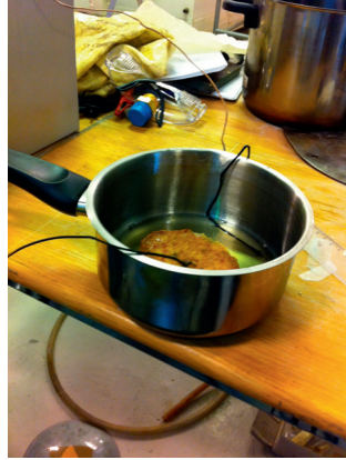
Figure 7: Installation of the thermocouple in the pan
