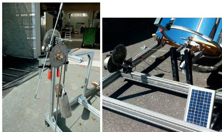
Figure 2.2.: Mechanical and electronic tracking systems tested
