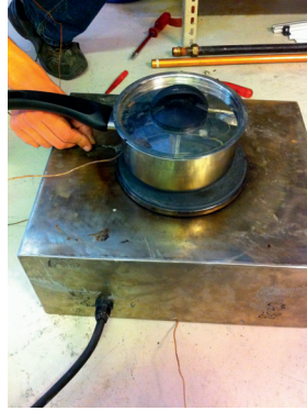
Figure 5: Modified heating plate - Constant temperature
