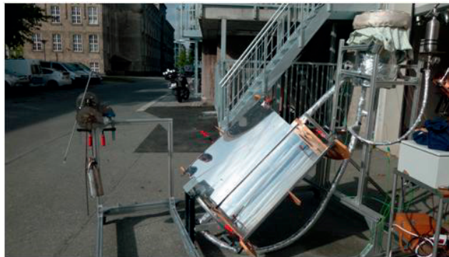
Fig. 1. Small-scale low-cost parabolic trough with heat storage for cooking purposes
