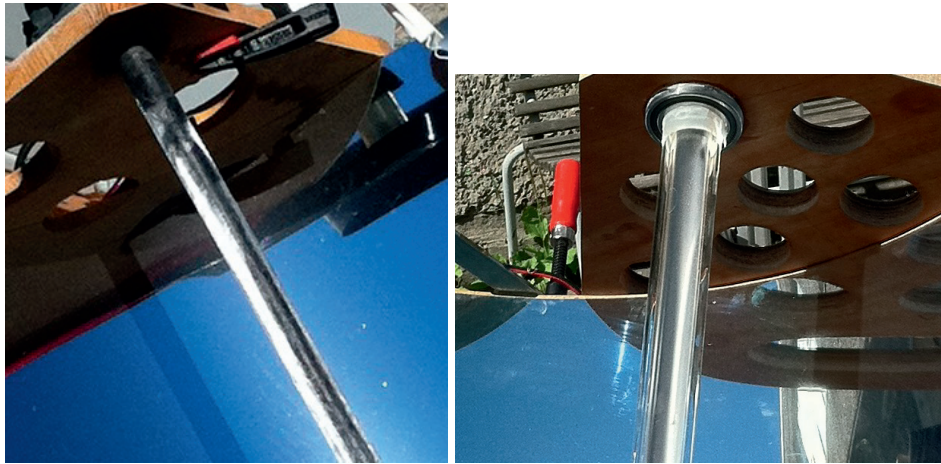
Figure 2.5.: Absorber without and with insulation
