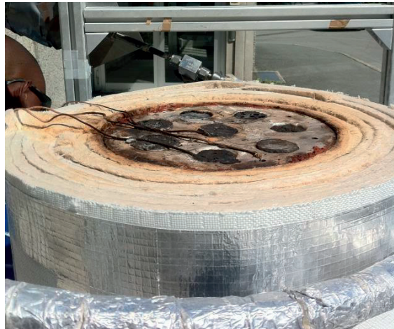
Fig. 2. View of the top of the storage – Aluminum and salt cylinders
