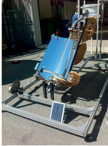
Figure 2: Heat storage-based system with parabolic trough
