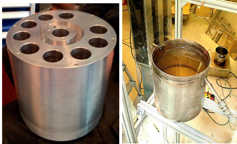
Figure 2.4.: Aluminum and oil-based storage structure
