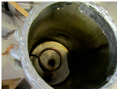
Figure 2.3.: Spiral running inside the storage
