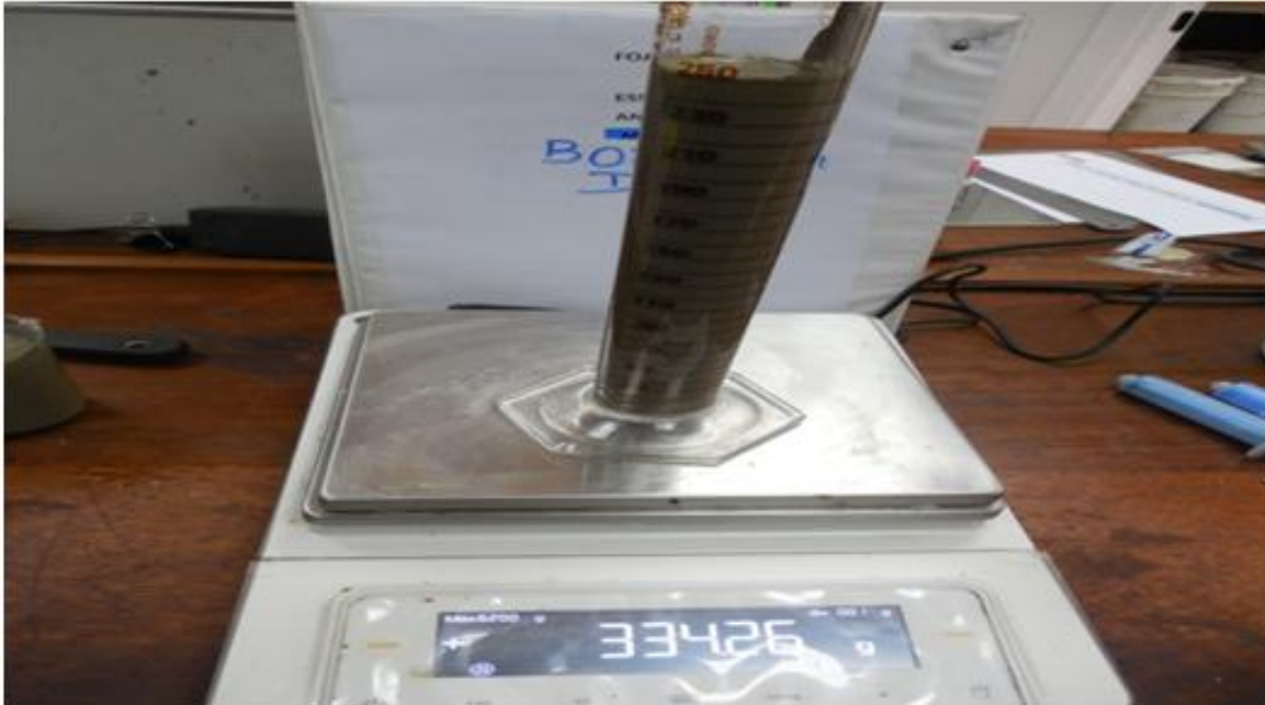
Figure 14: Graduated cylinder for unset foam test (Courtesy of Baker Hughes Cementing Laboratory-Angola)
