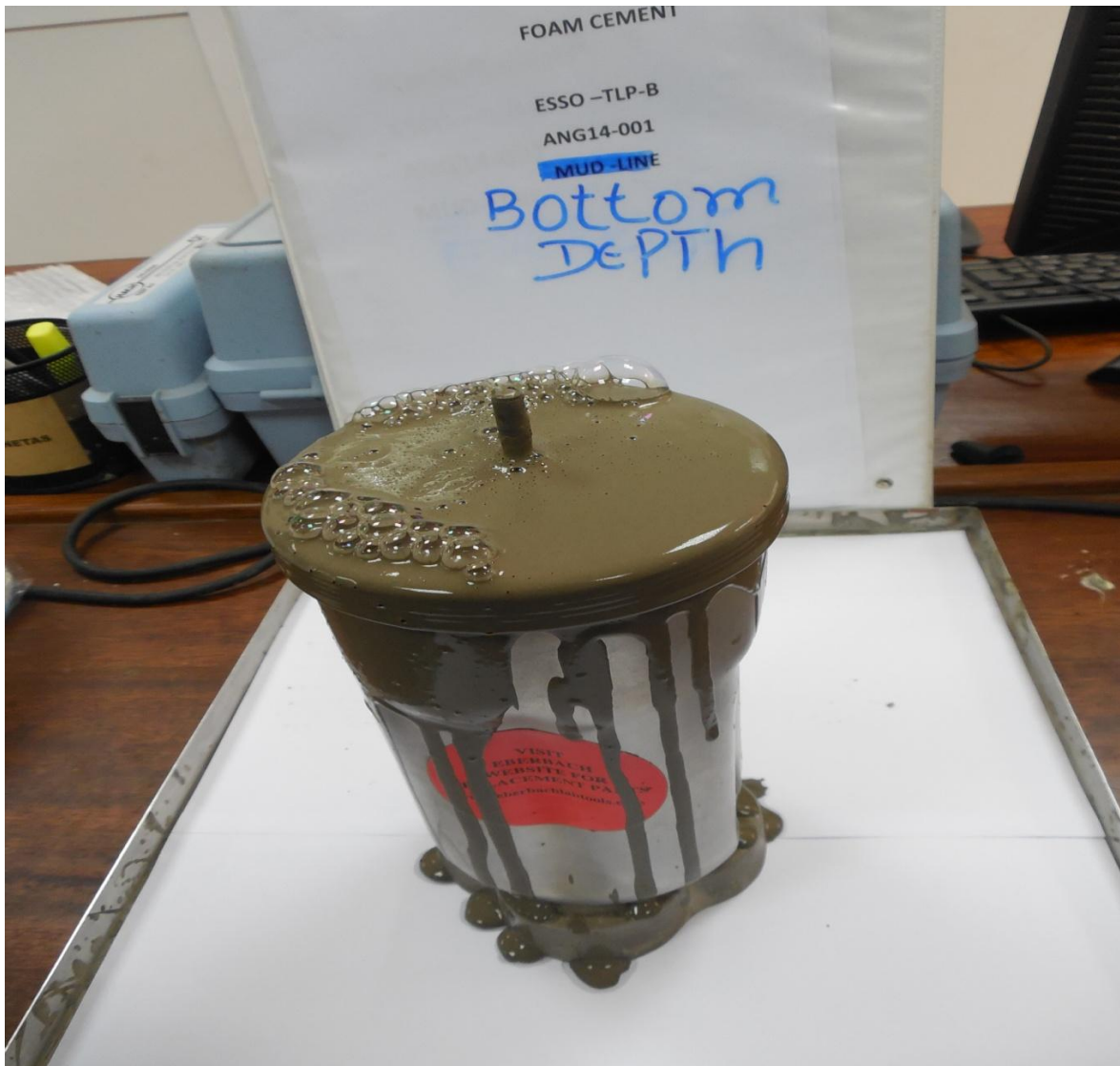
Figure 11: Slight pressure in the blending container due to temperature increases (Courtesy of Baker Hughes-Angola)
