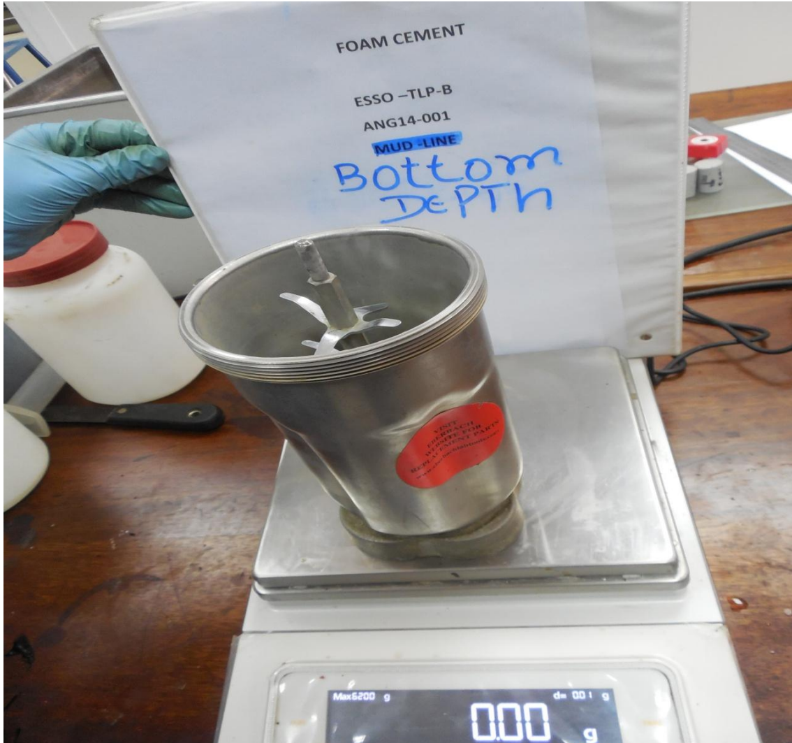
Figure 9: Blending container and multi-blade assembly ( Courtesy of Baker Hughes)
