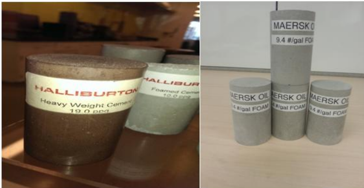
Figure 15: Curing mold for set cement test (Courtesy of Halliburton Cementing Laboratory)
