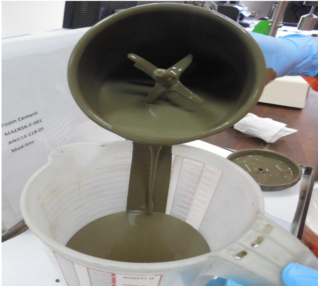
Figure 12: Check up of the cement slurry (Courtesy of Baker Hughes-Angola)
