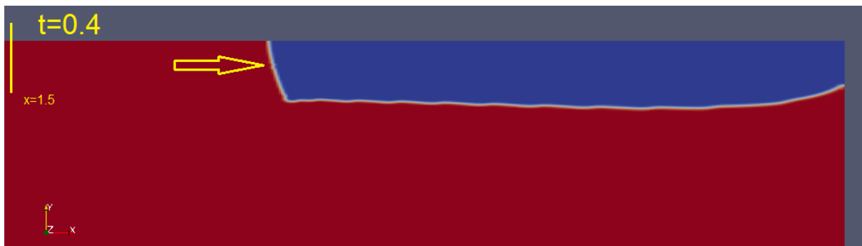
Figure A.37: Case 1 first time-step of diffusion, with PISO and nCorrectors=10
