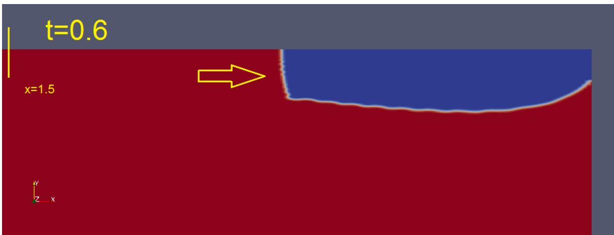
Figure A.36: Case 1 first time-step of diffusion, with PIMPLE instead of PISO
