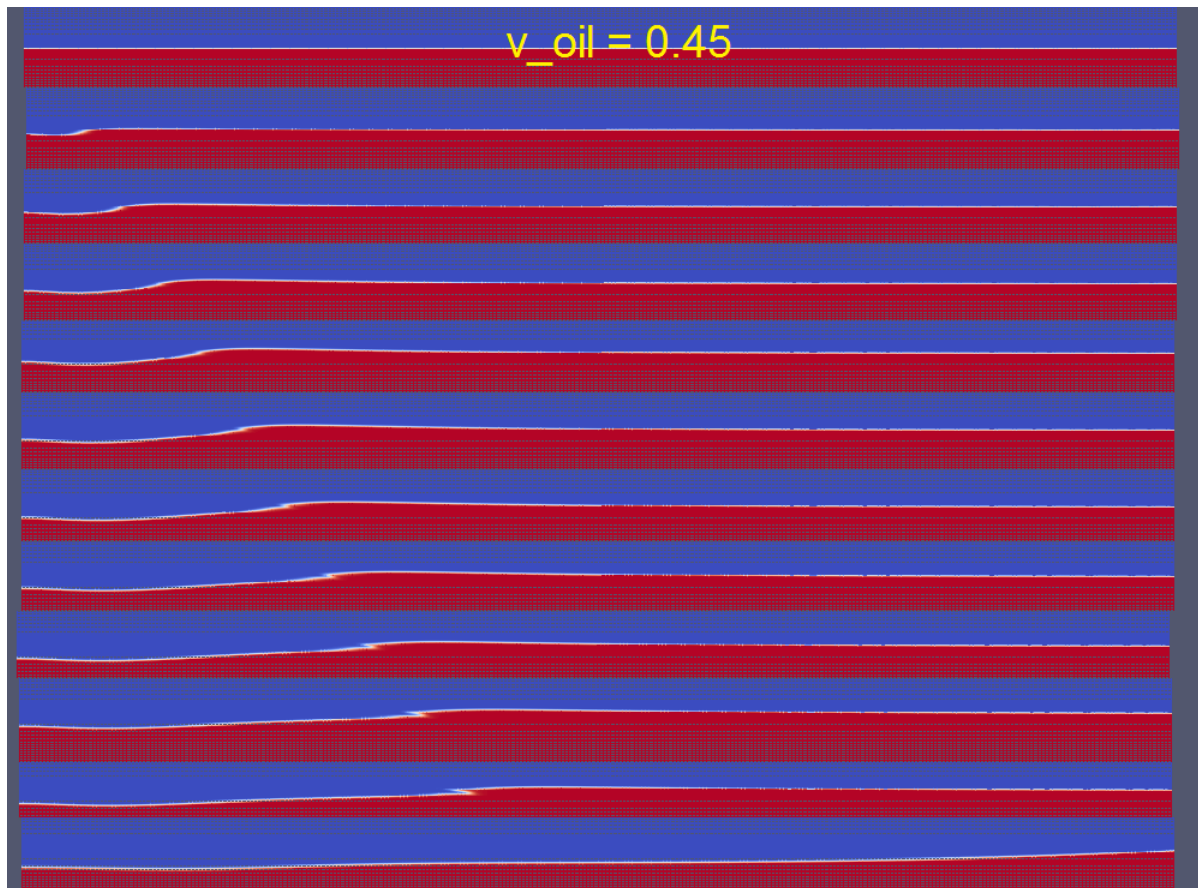
Figure 8.18: Flow pattern for case with v_{oil} = 0.45
