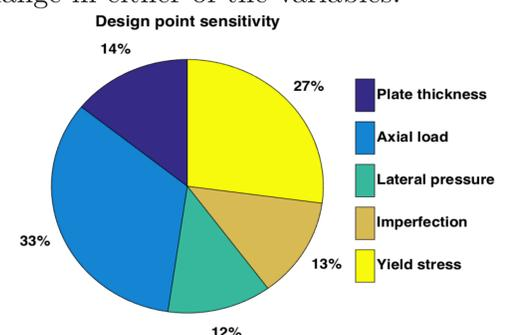
From the quadratic limit state, simulations were performed by the Crude Monte Carlo and Importance Sampling method. The results were similar to the results using FORM.
