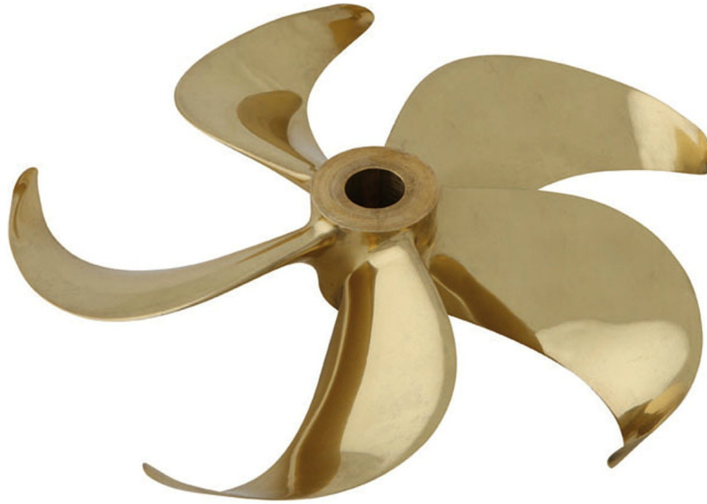
Figure 1.4: A 1:28 scale model of a Kappel Alpha 6.4 m diameter propeller (The Motorship 2012b).
