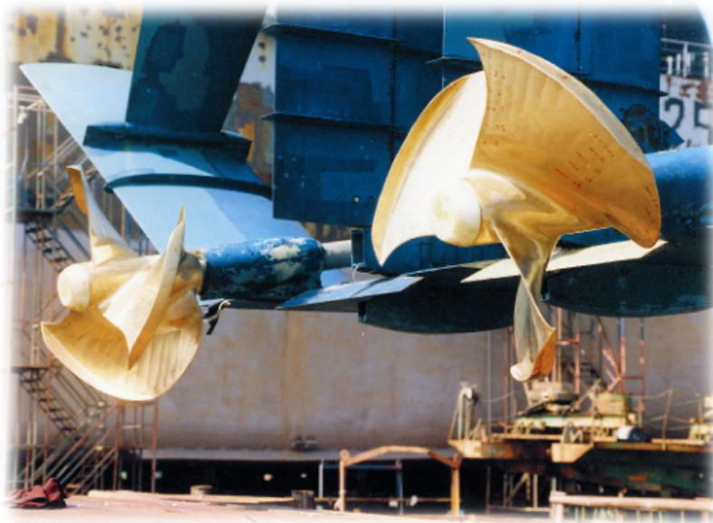
Figure 1.3: A hydrofoil vessel fitted with two fixed pitch CLT propellers (Gonzalez-Adalid and Gennaro 2011).
