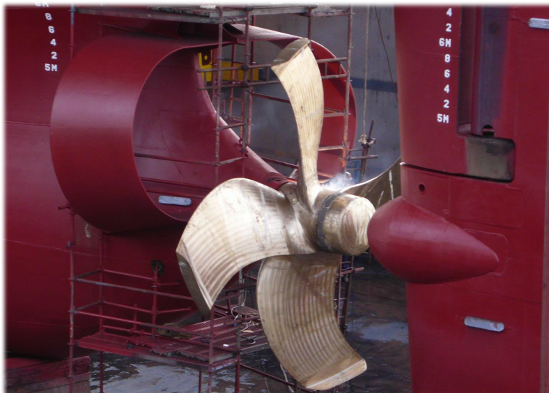
Figure 1.2: A 5.25 m diameter fixed pitch CLT propeller installed behind a wake equalising duct on the tanker M/T ‘Roy Maersk’ of A.P. Møller – Mærsk (The Motorship 2012a).
