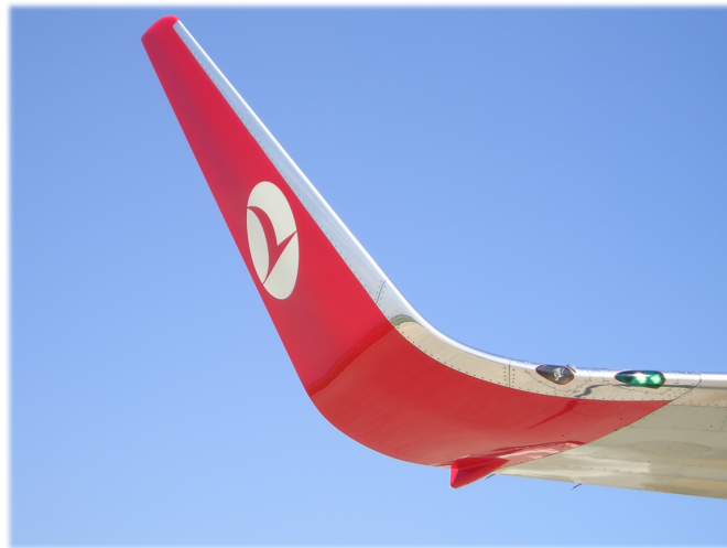
Figure 1.5: The blended winglet of a Boeing 737-800 (Wikimedia Commons 2007).
