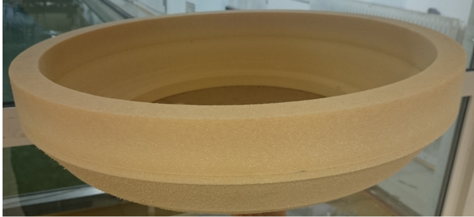
Figure 4.5: Foam ring milled from Divinycell H60.
