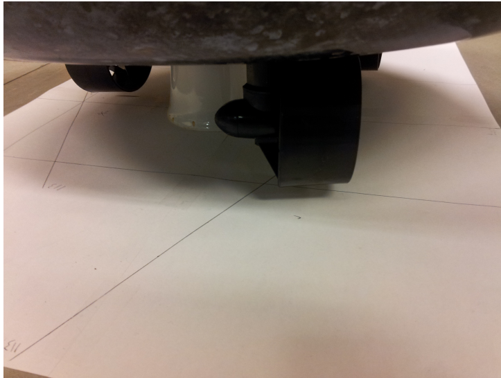
Figure 6.1: Paper template used to determine the maximum rotation of the thrusters.
