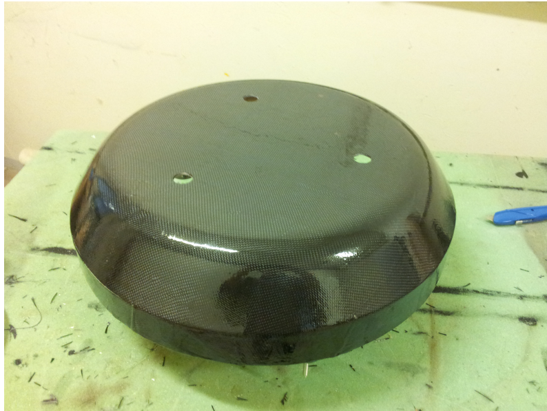
Figure 4.8: Vessel hull with exterior carbon coating.
