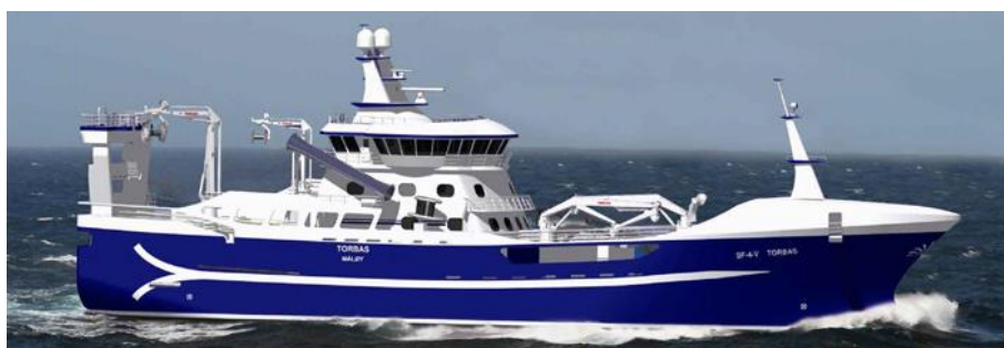
Figure 2-2 - Torbas. Rear/mid mounted superstructure (Seacon, 2014)
