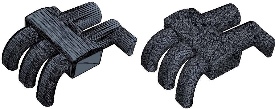
Figure 4-6 - Example of before and after remeshing (CD-Adapco, 2014)
