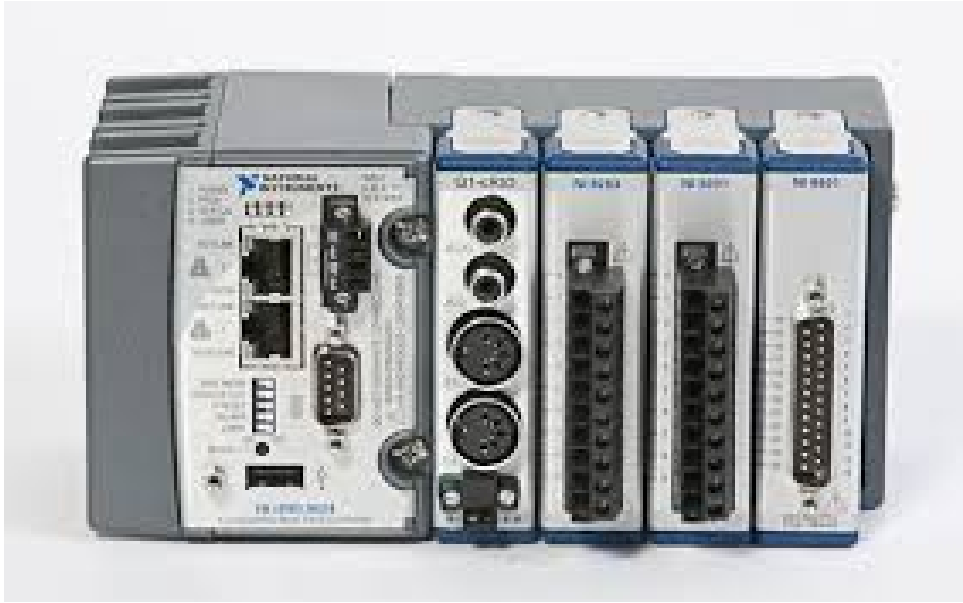
Figure 2.4: CompactRIO-9024 (courtesy: National Instruments (2015))
