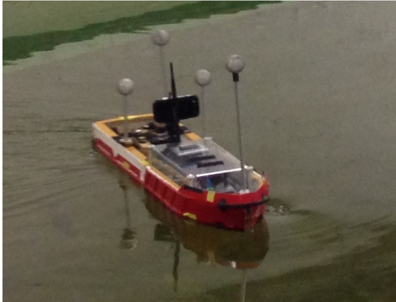
Figure 2.8: CSE1 fitted with mobile phone camera system
