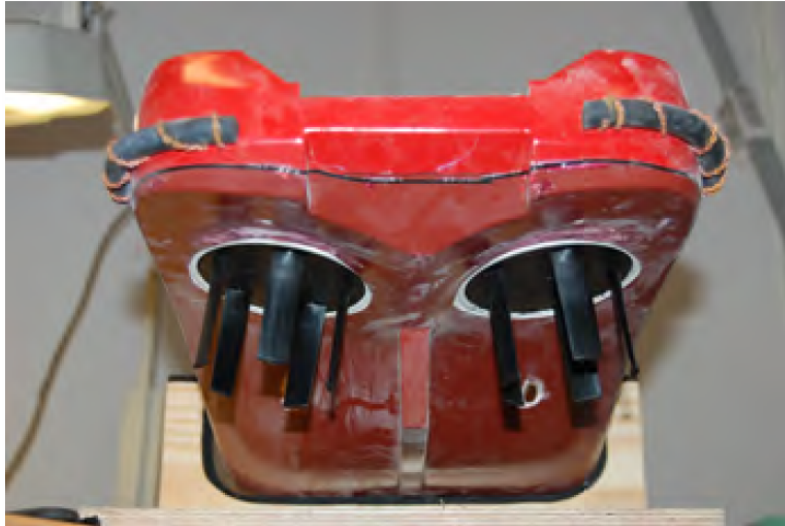
Figure 2.7: VSP propellers from as installed in CSE1 (courtesy: Skåtun (2011))
