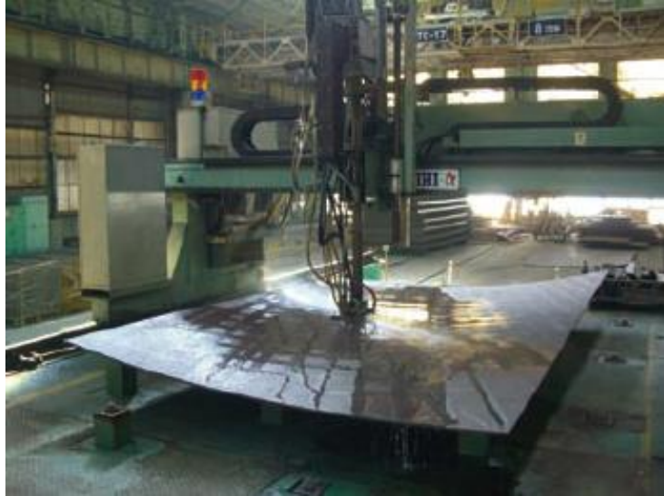
Figure 15 - Automatic heat-line system called "IHIMU-alpha". Source: : (Yoshihiko, 2011).
