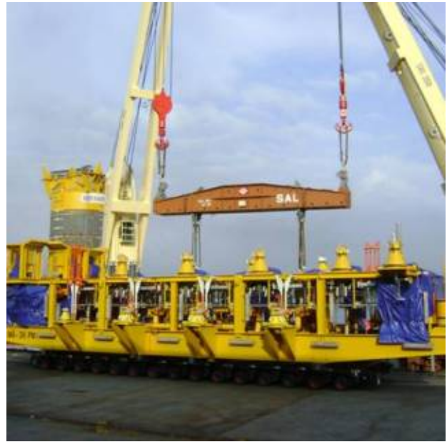
(b) Deepwater cluster manifolds from AkerSolutions ( AkerSolutions, 2014b )
