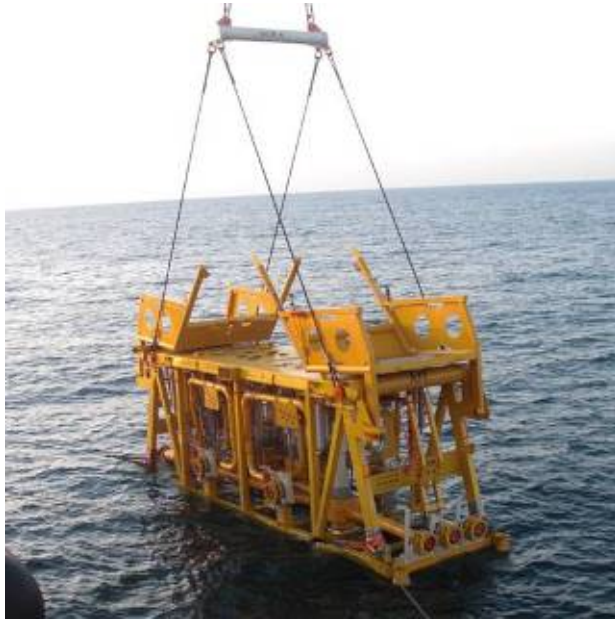
(a) Small manifolds system from AkerSolutions ( AkerSolutions, 2014e )
