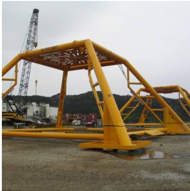
(c) Satellite protection structure from AkerSolutions ( AkerSolutions, 2014d )
