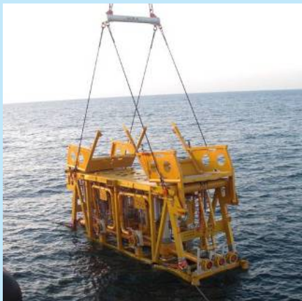
Manifolds are often in system with each other, protected by a tubular frame. AkerSolutions (2014b)
