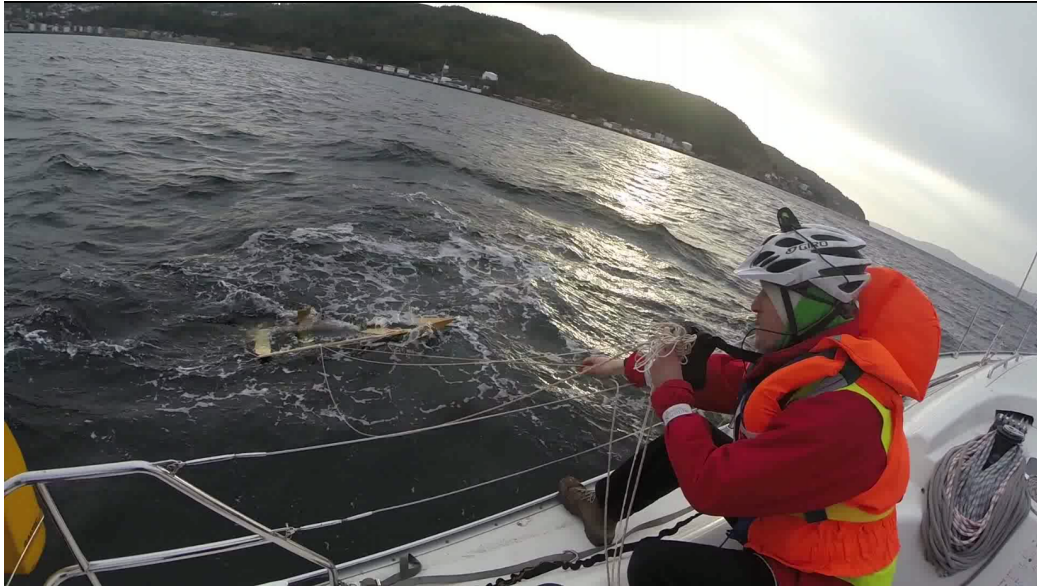
Figure 3.10: Tow test of 1 st paravane design iteration
