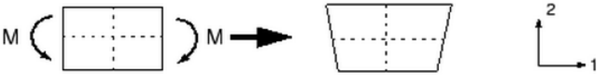
Figure 7.2 – Bending of linear element with reduced integration subjected to bending moment M.
