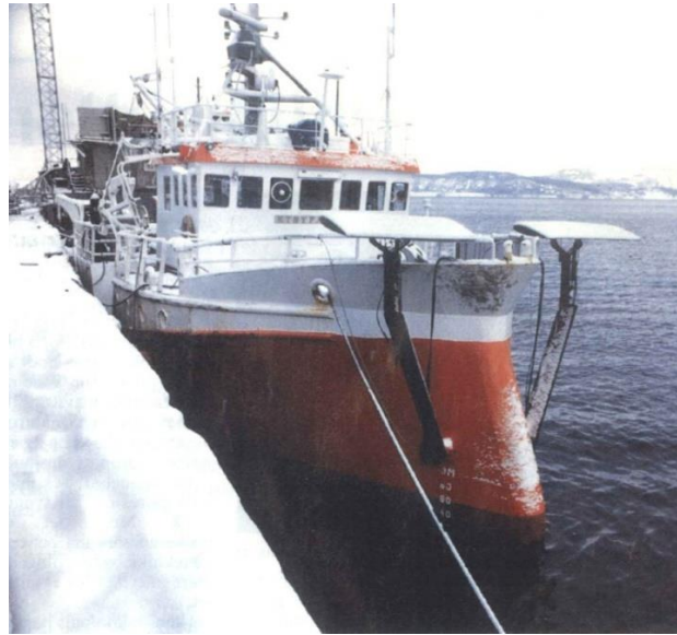
Figure 1-5: View of the foils fixed to struts in the bow of fishing vessel Kystfangst (Dybdahl, 1988)
