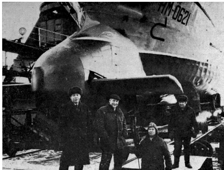
Figure 1-6: Russian trawler with bow-mounted wave foils (Nikolaev, 1995)
