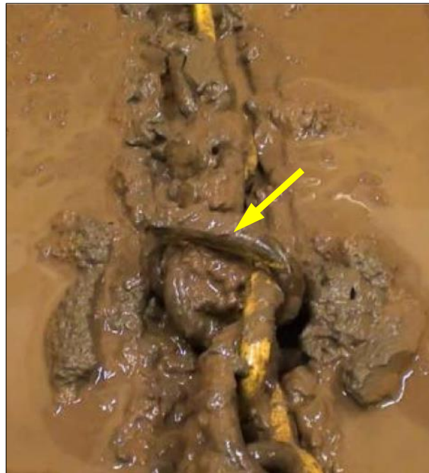
Figure 5-7: Twist in chain appearing in clay model test during chain pulling (Total, 2014).
