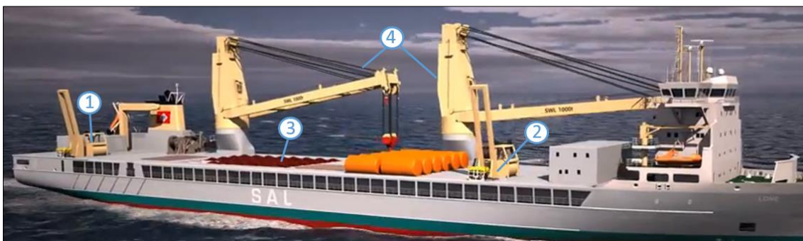
Figure 3-6: Heavy lift MV “Lone” equipped for DPA installation (SAL Heavy Lift, 2013).
