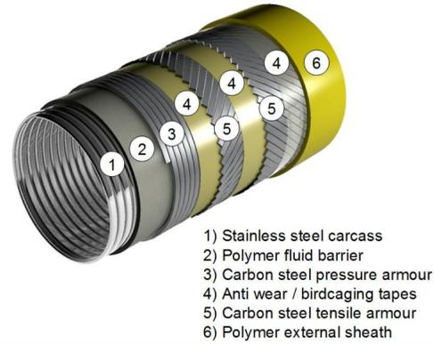
A flexible pipe is terminated with an end fitting where all layers are anchored and clamped in a special end structure. To limit the bending stresses and excessive curvature a bend stiffener is added to improve the stiffness of the flexible pipe which connecting the end fitting. There are two kinds of flexible pipes which named as bonded and non-bonded pipe. For non-bonded pipes, the cylindrical layer is able to slide relative to adjacent layers.
