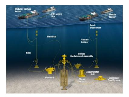
Figure 2-1 A typical flexible pipe system, Image: MWCC
