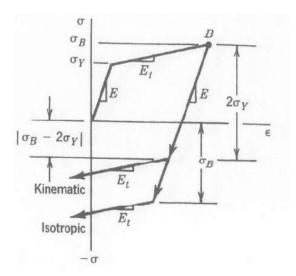
Figure 3-23 kinematic hardening and isotropic hardening
