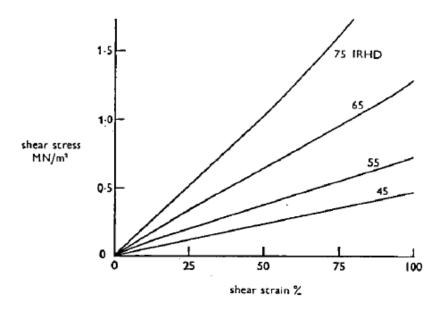
Figure 2-6 The strain-stress curves of rubber in shear deformation
