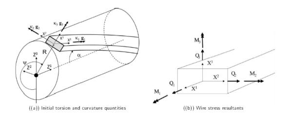
Figure 3-11 Definition of wire coordinate axes and the mechanical quantities
