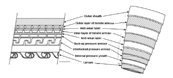
Figure 2-3 Typical non-bonded flexible pipe cross-section
