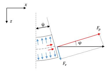
Figure 3-7 Equilibrium of the forces  $F_{\nu}$  and  $F_{p}$ , under assumption of no ovalization
