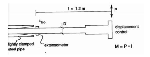
Figure 4-12 Test set-up of the sample bonded flexible pipe
