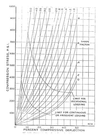
Figure B-4 Compression of solid rubber rings
