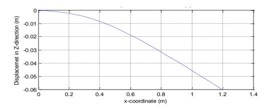
Figure 4-8 Global displacement of the non-bonded pipe
