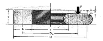
$$K = \frac{F}{x} = \frac{4}{3} \frac{E_0 \pi (D^2 - d^2)}{4t} \left\{ 1 + k \left( \frac{D - d}{4t} \right)^2 \right\}$$
