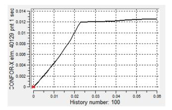
Figure 4-7 Longitudinal contact force on a typical contact element
