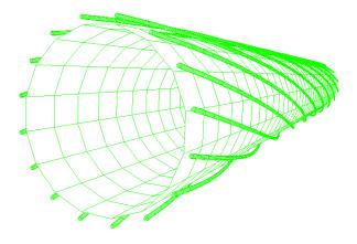
Figure 5-4 FE model of the inner tube and helical tendons of umbilical
