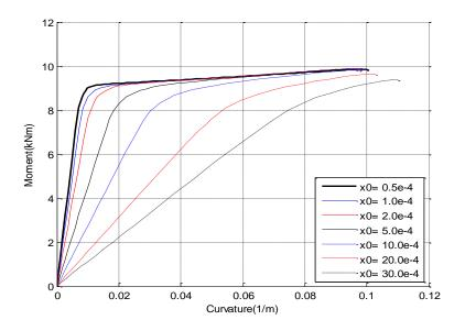
Figure 5-29 Moment-curvature result in parameter study on the shear stiffness
