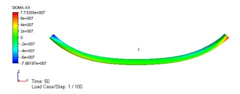
Figure 5-21 Global distribution of the longitudinal stress  $\sigma_{xx}$
