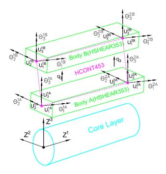
Figure 3-20 DOFs system of HCONT453 element
