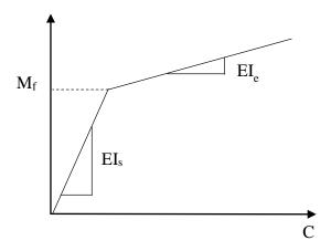
Figure 3-13 Typical moment curvature relation for non-bonded flexible pipe
