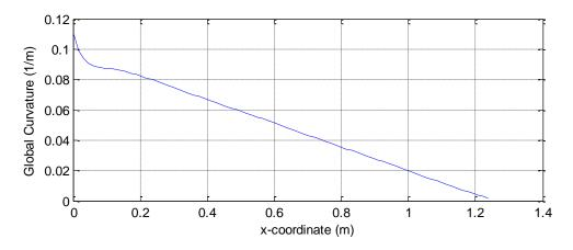
Figure 4-21 Global curvature of the PIPE31 bonded flexible pipe model
