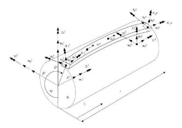
Figure 3-18 The dofs system of HSHEAR353 element
