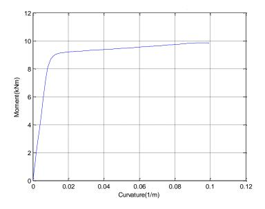
Figure 5-11 Moment-curvature of umbilical middle section
