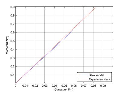
Figure 4-19 Moment-curvature plots of the PIPE31 model and Pag-o-flex sample pipe
