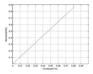
Figure 4-25 Moment-curvature of the HSHEAR363 model
