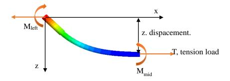
Figure 5-8 Equilibrium of the umbilical at the measurement location
