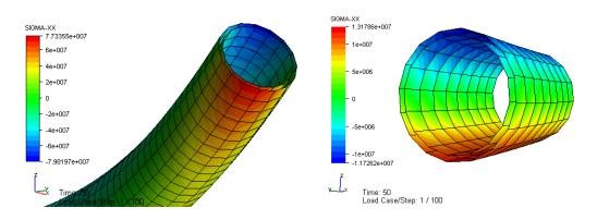
Figure 5-22 Longitudinal stress  $\sigma_{xx}$  at the end region and middle section, inner tube and outer sheath
