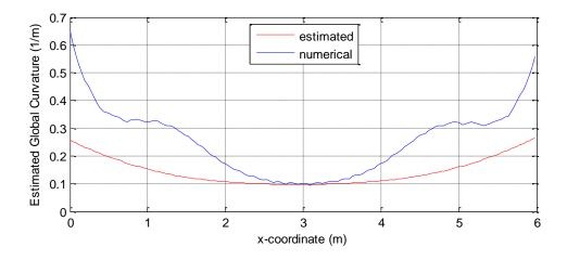
Figure 5-17 Global curvature from numerical result and estimation
