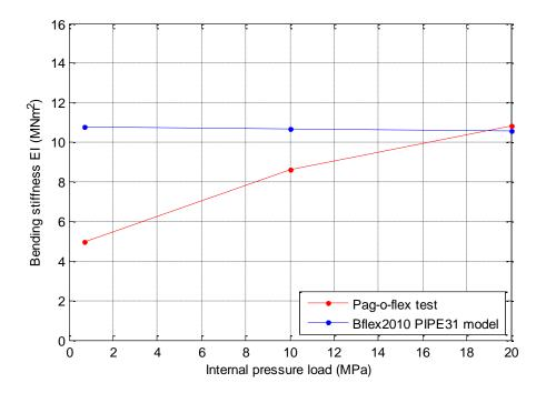
Figure 4-24 Effect of internal pressure on EI, in PIPE31 model
