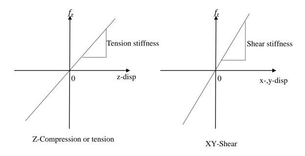
Figure 4-14 Illustration of tension stiffness and shear stiffness
