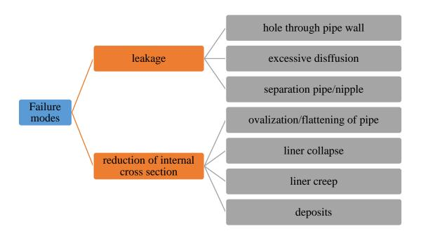
Figure 2-2 Failure modes of flexible pipes
