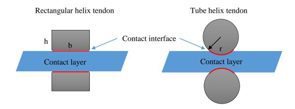
Figure 4-16 Illustration of the contact interface width
