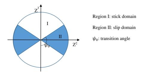
Figure 3-14 Cross-section stick and slip domain
