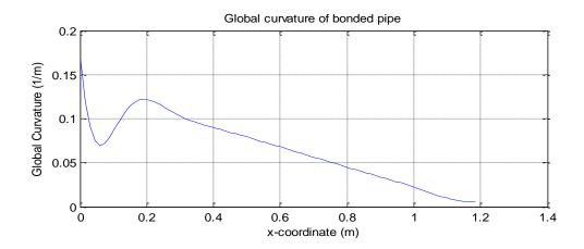
Despite of the significant end effect, the measure point successfully avoids this uncertainty. The curvature decreases smoothly to zero between the 0.4 m to 1.2 m.
