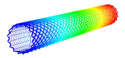
Figure 4-2 FE model of the non-bonded flexible pipe
