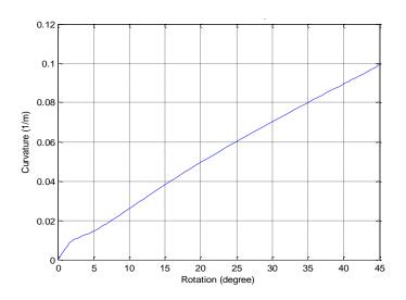
Figure 5-9 Curvature of the umbilical middle section
