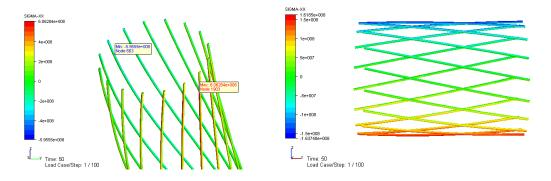
Figure 5-23 Longitudinal stress  $\sigma_{xx}$  at the end region and middle section, tensile layer
