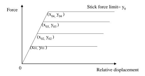
Figure 5-32 Threshold model of stick limit in the parameter study
