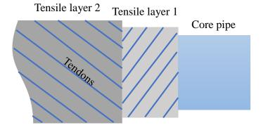
Figure 4-1 Illustration of the non-bonded flexible simplified model
