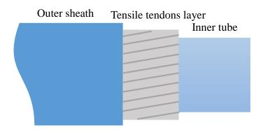
Figure 5-1 Main structural components of umbilical model
