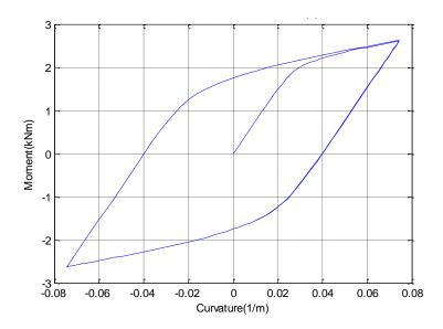
Figure 4-10 Moment-curvature of non-bonded pipe at cyclic loading
