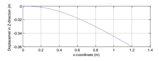
The displacement constraint is applied at the right end, making the sectional moment increases linearly to its maximum at the clamped left end. If assuming consistent bending stiffness along the pipe length, the curvature would also show the same trend like the sectional moment.
