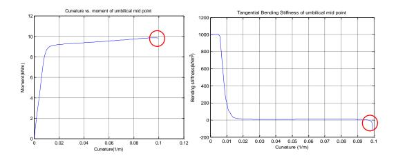
Figure 5-37 End effect error caused by numerical simulation
