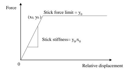
Figure 2-10 Slip threshold model of bitumen contact layer
