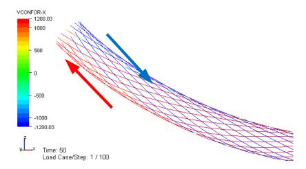
Figure 5-26 Distribution of the contact force in local x direction
