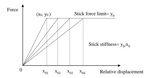
Figure 5-28 Threshold model of shear stiffness in the parameter study
