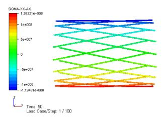
Figure 5-24 Axial stress on the tendons at the middle section
