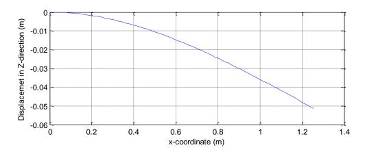
Figure 4-20 Global deflection of the PIPE31 bonded flexible pipe model
