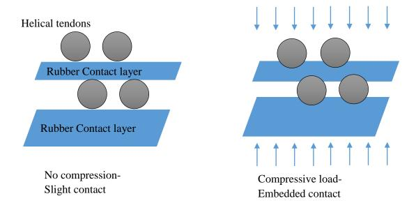
Figure 3-5 Compression model for rubber contact layers
