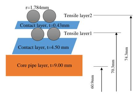
Figure 4-17 Cross section of the bonded flexible pipe model
