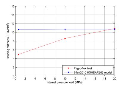
Figure 4-29 Effect of internal pressure on EI, in HSHEAR363 model
