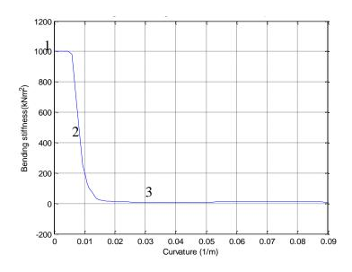
Figure 5-12 Tangential bending stiffness history, divided into three phases
