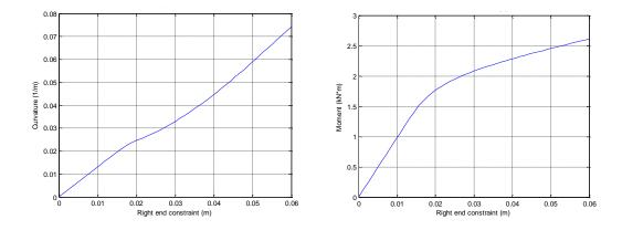
Figure 4-5 Curvature and moment history of the non-bonded flexible pipe
