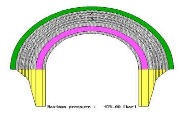
Figure 3-4 Pressure distribution in a typical flexible pipe exposed to internal pressure [1]
