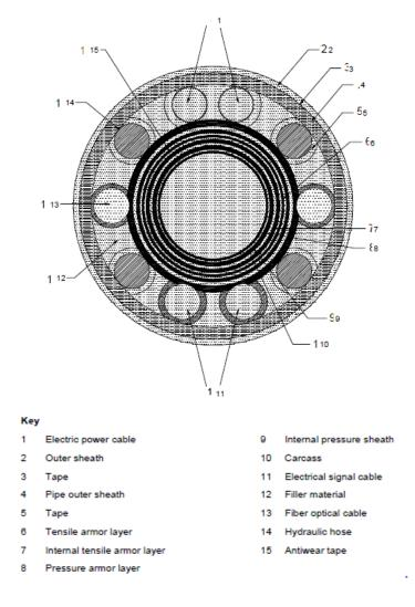
Figure 2-9 Typical configuration of umbilical pipe
