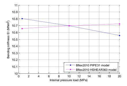
Figure 4-30 Comparison of the effects of internal pressure on EI from two models
