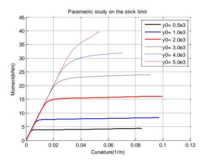
Figure 5-33 Moment-curvature result in parameter study on the stick limit
