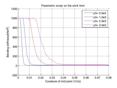
Figure 5-34 Tangential EI in parameter study on the stick limit
