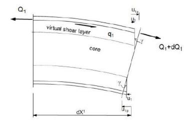
Figure 3-16 Shear deformation model [1]
