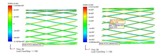
Figure 5-25 Distribution of longitudinal stresses due to bending, middle section
