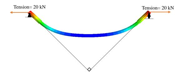
Figure 5-6 Boundary condition and angle constraint of the umbilical
