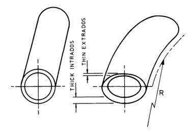
Figure 3-8 Ovalization of pipe after bending [12]
