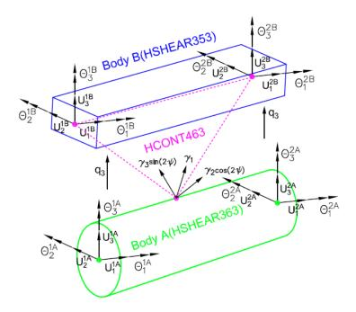
Figure 3-21 DOFs system of HCONT463 element, image
