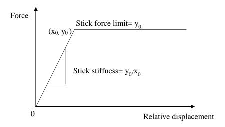
Figure 5-5 Stick-slip model of the bitumen contact material
