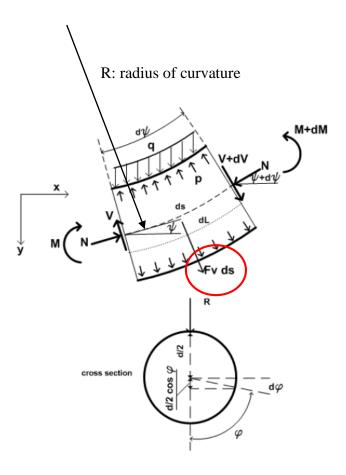
Figure 3-6 Equilibrium of an infinitesimal pipe segment, assuming constant circular cross section [11]
