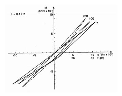
Figure 4-13 Moment-curvature curves at different internal pressure levels of Pag-oflex sample pipe [19]
