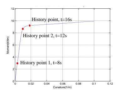
Figure 5-18 Selection of history points on the moment-curvature curve
