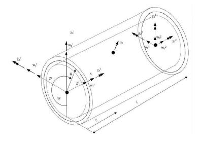
Figure 3-19 The Dofs system of HSHEAR363 element
