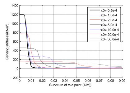
Figure 5-30 Tangential EI in parameter study on the shear stiffness
