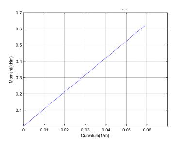
Figure 4-18 Moment-curvature of the PIPE31 bonded flexible pipe model
