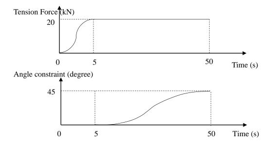
Figure 5-7 Load history of the simulation of umbilical
