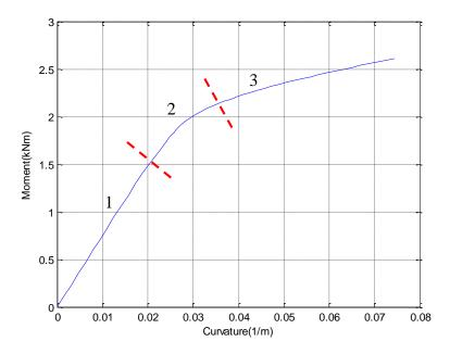
Figure 4-6 Moment-curvature of non-bonded flexible pipe
