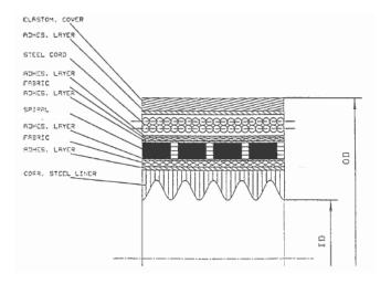
Figure 4-11 Detail section of the Pag-o-flex sample pipe [19]
