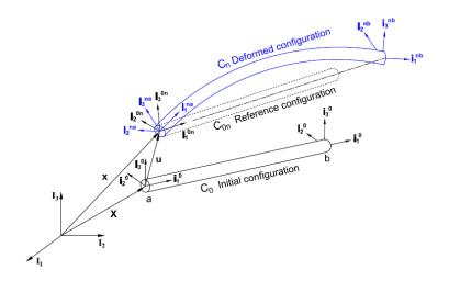
Figure 3-17 Motion of beam nodes [17]
