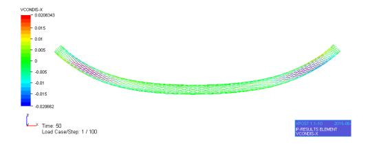
Figure 5-27 Distribution of the relative displacement in local x direction
