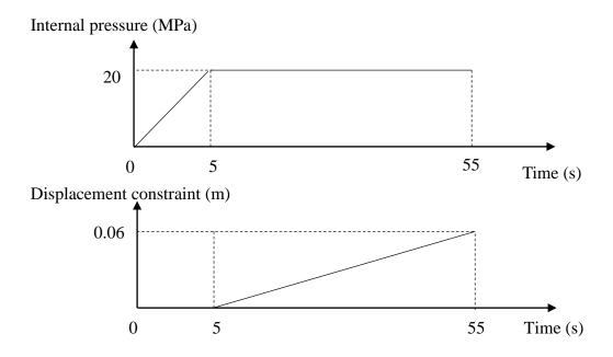
Figure 4-4 Loading history of the internal pressure and the displacement constraint
