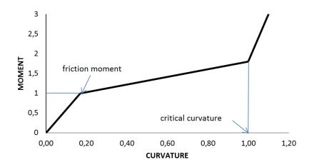
Figure 2-4 Bending behavior of non-bonded pipes [3]
