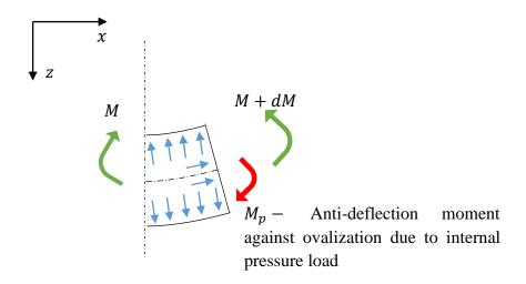
Figure 3-10 Anti-deflection moment, in case of pipe ovalization
