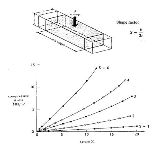
Figure 2-7 Typical compression stress-strain curve for strip rubber
