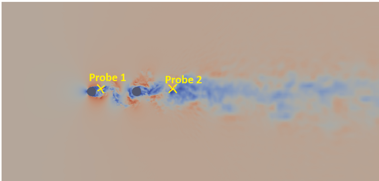
Figure 5.11: Probe locations marked in the computational domain with coloring of velocity U
