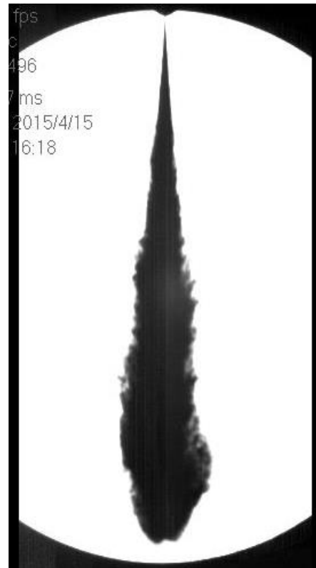
Figure 20: Shadowgraph Imaging Technique
