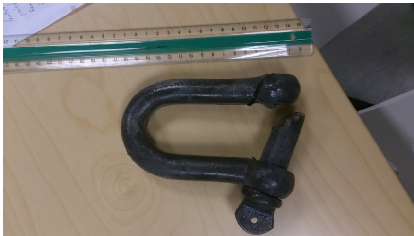
Figure 3.7: Failed chain link. PHOTO: Bi-Brygga AS
