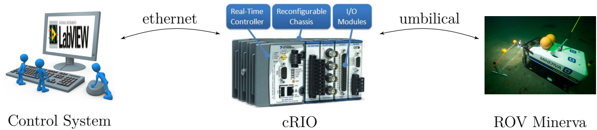
Figure 3.4: Illustration of the hardware structure for the ROV Minerva control system. Pictures with courtesy: PC , Puzzledworld; cRIO + Logo , NI; Minerva , TU.
