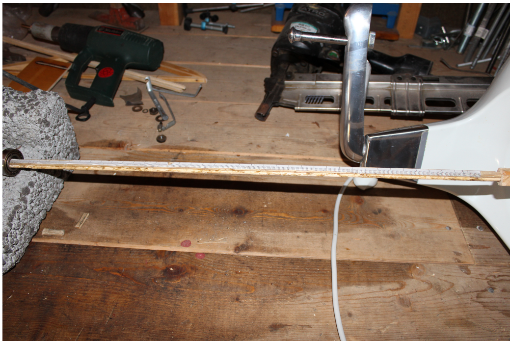
Figure 6: The shaft that the fishing lined was spooled onto with scale marking the distance between each tread
