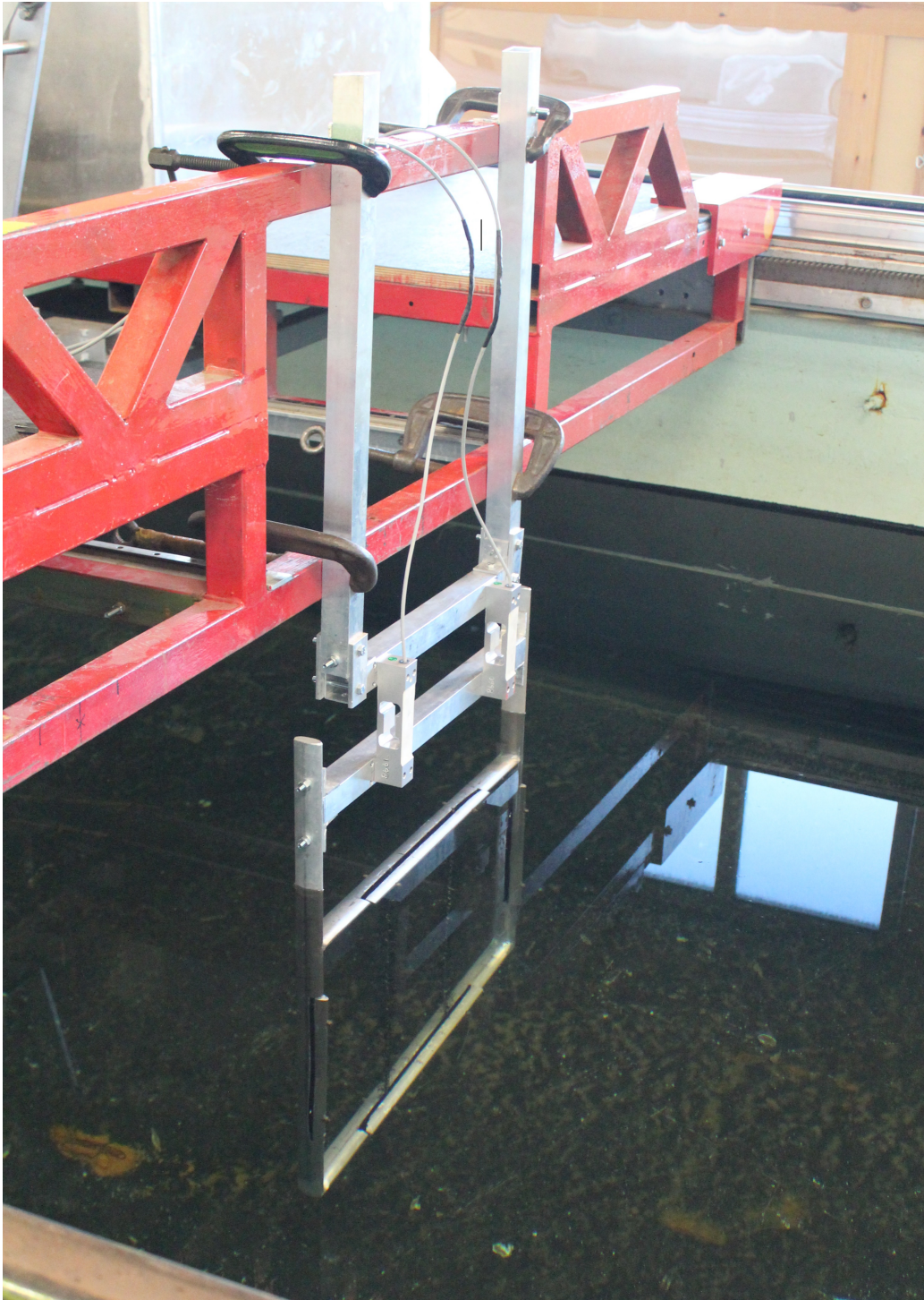
Figure 9: The complete frame rig mounted on the towing carriage
