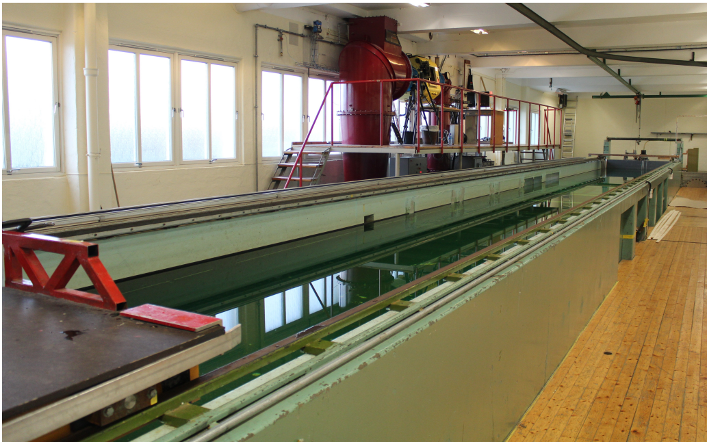
Figure 7: The small towing tank at MarinTek, Tyholt
