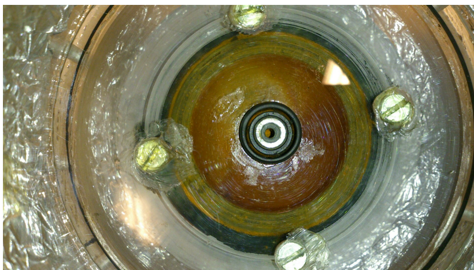
Figure 24 – Picture of the newly washed photoreactor. When it was flushed with ethanol and wiped with a white paper, the paper turned black, proving that this is likely to be a contamination source.
