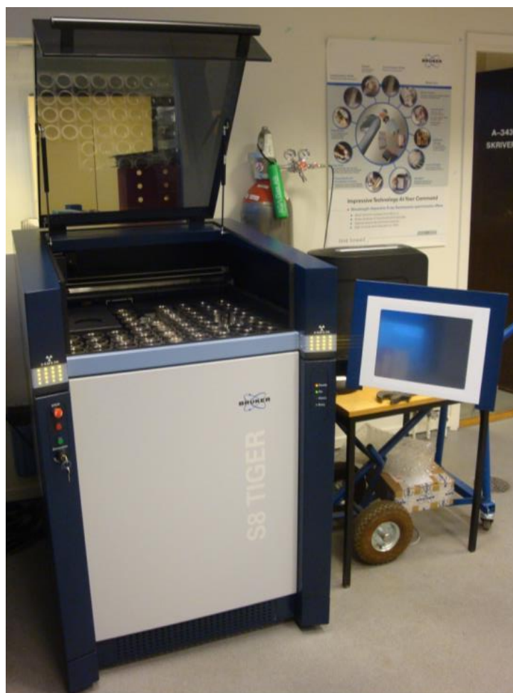
Figure 4-3: The S8 TIGER machine that was used for the XRF chemical analysis.
