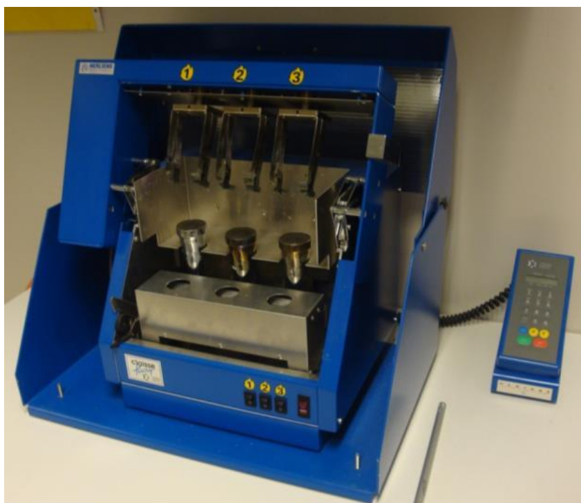
Figure 4-4: The Caisse Fluxy fusion device that was used.
