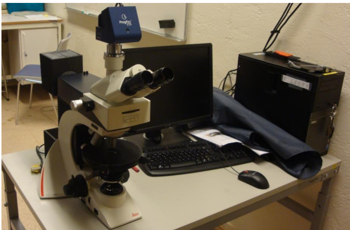
Figure 4-2: The Leica DM2500 P optical microscope that was used to identify minerals in thin sections.
