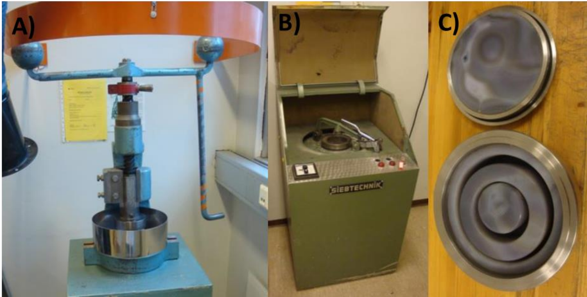
Figure 4-1: A shows the Fly press rock crusher that was used to crush the samples. B shows the Disk mill which the agate mill (shown in C) was inserted into.
