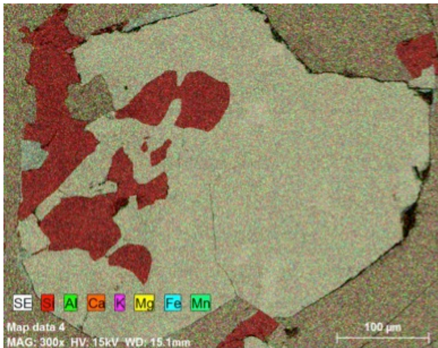
Figure 22: Element map reveals that there is no internal zonation within the garnet. The slightly brighter grey areas within the garnet are due to charging of the sample.
