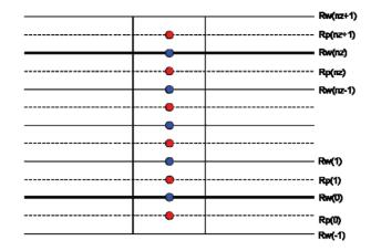
FIGURE 2.2. Computational grid in wall-normal direction. Red and blue circles represent the cell-centers and cell-faces, respectively.
