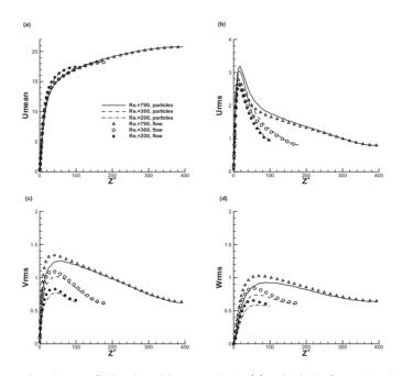
Figure 6: Comparison between fluid and particle mean velocity (a) and velocity fluctuations in the streamwise (b), spanwise (c), and wall-normal (d) directions for  $\tau^+=5$ . The symbols denote fluid velocities and the lines represent particle velocities. The profiles are terminated at the mid-plane of the channel.
