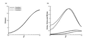
Figure 3: Streamwise mean particle velocity (a) and RMS velocity fluctuations (b) for  $\tau^+{=}30$
