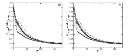
FIG. 5. Comparison between fluid spin intensities  $\Omega_{y,rms}$  (symbols), conditionally averaged fluid spin intensities  $\Omega_{y,rms}^{P}$ (lines), and particle spin intensities  $\omega_{y,rms}^{P}$ (lines),  $\tau_{t}^{+} = 1$ : triangle and solid line;  $\tau_{t}^{+} = 5$ : open circle and dashed line;  $\tau_{t}^{+} = 30$ : square and dash dot line. (a) fluid and particles and (b) fluid and conditionally averaged fluid at particle positions.
