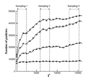
Figure 1: Development of particle concentration in the near-wall region  $z^+ < 12$  for  $Re_*=200$ . The double arrows show three different sampling periods each of duration 2820 viscous time units.  $\tau^+=1$ , squares;  $\tau^+=5$ , triangles;  $\tau^+=30$ , diamonds;  $\tau^+=100$ , circles.
