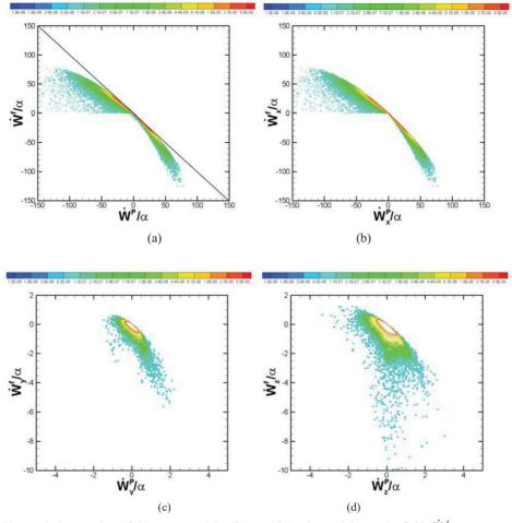
Figure 13. Scatter plots of the power resulting from work by the particles on the fluid  $\dot{W}^{f}$  versus power resulting from work by the fluid on the particles  $\dot{W}^{P}$ . (a) Total powers. Events on the straight line  $\dot{W}^{f} = -\dot{W}^{P}$  corresponds to  $\varepsilon_{P} = 0$ . (b) Power exchange due to streamwise motions; (c) power exchange due to wall-normal motions; (d) power exchange due to spanwise motions. Notice the different scaling in the two lower panels.
