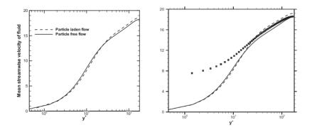
FIG. 1. Left: mean streamwise velocity of the fluid in present simulation. Right: mean streamwise velocity of the fluid in Dritselis and Vlachos<sup>1</sup>. Continuous line: fluid velocity of particle-free flow; dashed line: fluid velocity of particle-laden flow; symbols: particle velocity.
