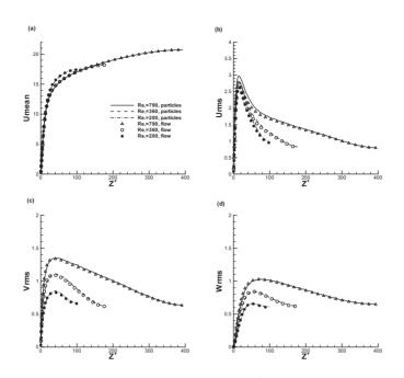
Figure 5: Comparison between fluid and particle mean velocity (a) and velocity fluctuations in the streamwise (b), spanwise (c), and wall-normal (d) directions for  $\tau^+=1$ . The symbols denote fluid velocities and the lines represent particle velocities. The profiles are terminated at the mid-plane of the channel.
