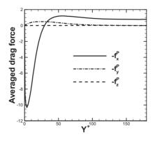
Figure 5 Profiles of the directional components of the averaged drag force  $-\overline{f_i^P}$ .
