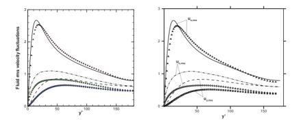
FIG. 2. Left: turbulence intensities of the fluid in present simulation. Right: turbulence intensities of the fluid in Dritselis and Vlachos<sup>1</sup>. Lines: particle-free flow; symbols: particle-laden flow.
