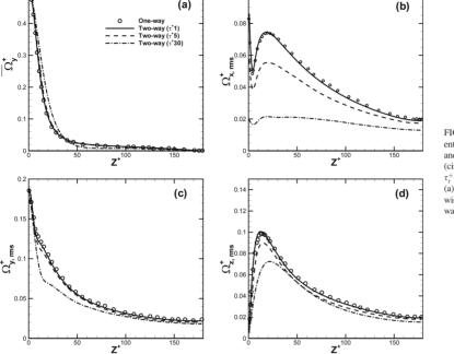
FIG. 2. Fluid spin. Results from the present two-way coupled simulations (lines) and the one-way coupled simulation (circles) by Mortensen et al. (Ref. 27).  $\tau_t^+ = 1$  -----;  $\tau_t^+ = 5$  -----;  $\tau_t^+ = 30$  -----(a) mean spanwise spin, (b) rms streamwise spin, (c) rms spanwise spin, (d) rms wall-normal spin.
