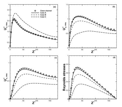
FIG. 1. Turbulence intensities and Reynold shear stress  $-u_{x}^{\prime}u_{z}^{\prime}$  for the twoway coupled simulations (lines) compared with data from a one-way coupled simulation (circles). ( $\tau_{t}^{+} = 1$  ——;  $\tau_{t}^{+} = 5 - \cdots$ ;  $\tau_{t}^{+} = 30$  -.--).
