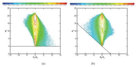
Figure 10. Scatter plot of streamwise velocity components. (a) Fluid velocity versus slip velocity; (b) particle velocity versus slip velocity. The straight lines in panels (a) and (b) are  $u_x = 0$  and  $v_x = -(u_x - v_x)$ , respectively.
