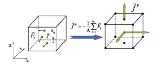
FIGURE 2.5. Illustration of point-particle forces  $\vec{F}_l$  transferred into volume force  $\vec{f}^P$  of fluid on the grid-nodes.
