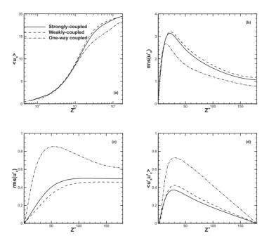
FIGURE 2. Flow-field statistics from the strongly-coupled simulation (solid lines) compared with results from the weakly-coupled simulation(broken lines). Results from a one-way coupled simulation (dash-dotted lines) are included for comparative purposes. (a) Mean streamwise velocity  $\langle u_x \rangle$ ; (b) streamwise turbulence intensity  $rms(u'_x)$ ; (c) wall-normal turbulence intensity  $rms(u'_z)$ ; (d) Reynolds shear stress  $\langle u'_x u'_z \rangle$ .
