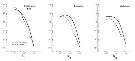
Figure 8 One-dimensional spectra of the fluid kinetic energy in the viscous sublayer at  $Y^+ \approx 6$  (a) Streamwise direction; (b) spanwise direction; (c) wall-normal direction.
