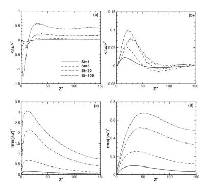
FIG. 2: Stokes number effects on mean and rms slip velocity statistics: (a-b) mean streamwise and wall-normal slip velocity,  $\langle \Delta u \rangle^+$  and  $\langle \Delta w \rangle^+$ ; (c-d) rms of streamwise and wall-normal slip velocity fluctuations,  $\langle rms(\Delta u') \rangle^+$  and  $\langle rms(\Delta w') \rangle^+$ .
