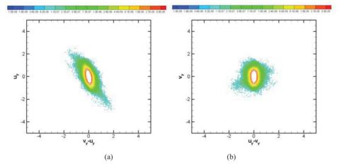
Figure 11. Scatter plot of wall-normal velocity components. (a) Fluid velocity versus slip velocity; (b) particle velocity versus slip velocity.
