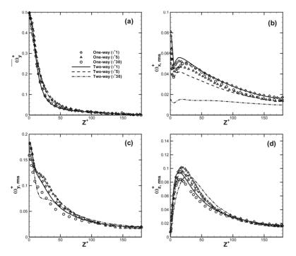
FIG. 3. Particle spin. Results from the present two-way coupled simulations (lines) and the one-way coupled simulations (symbols) by Mortensen *et al.* (Ref. 27).  $\tau_t^+ = 1$  —, diamond;  $\tau_t^+ = 5$  - - -, triangle;  $\tau_t^+ = 30$  -.-., circle (a) mean spanwise spin, (b) rms streamwise spin, (c) rms spanwise spin, (d) rms wall-normal spin.
