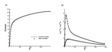
Figure 4: Mean streamwise fluid velocity (a) and velocity fluctuations  $\langle u^{+2} \rangle$ ,  $\langle v^{+2} \rangle$ (b). Results from the present simulation at  $Re_*$ = 790 (lines) are compared with DNS data from Abe et al. [19] [20] at the same Reynolds number.
