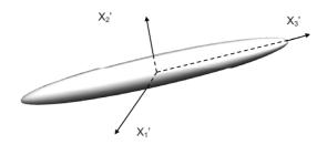
FIGURE 2.3. A schematic of a prolate spheroid with an aspect ratio of about to 5. The major or polar axis is aligned with the  $x'_3$ -direction in the particle coordinate system which has its origin in the center of the spheroidal particle.
