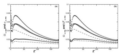
FIG. 4. Comparison between fluid spin intensities  $\Omega_{x,rms}$  (symbols), conditionally averaged fluid spin intensities  $\Omega_{x,rms}^{P}$  (lines), and particle spin intensities  $\omega_{x,rms}$  (lines).  $\tau_{t}^{+} = 1$ : triangle and solid line;  $\tau_{t}^{+} = 5$ : open circle and dashed line;  $\tau_{t}^{+} = 30$ : square and dashed dotted lines. (a) fluid and particles and (b) fluid and conditionally averaged fluid at particle positions.
