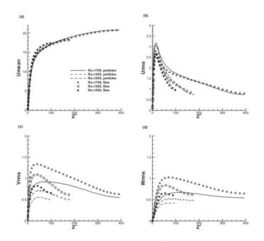
Figure 7: Comparison between fluid and particle mean velocity (a) and velocity fluctuations in the streamwise (b), spanwise (c), and wall-normal (d) directions for  $\tau^+$ =30. The symbols denote fluid velocities and the lines represent particle velocities. The profiles are terminated at the mid-plane of the channel.
