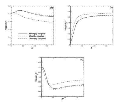
FIGURE 3. Mean particle orientation in the weakly- and strongly-coupled simulations. (a) Streamwise direction cosine  $|\cos\theta_x|$ ; (b) spanwise direction cosine  $|\cos\theta_y|$ ; (c) wall-normal direction cosine  $|\cos\theta_z|$ . Legend as in figure 2.
