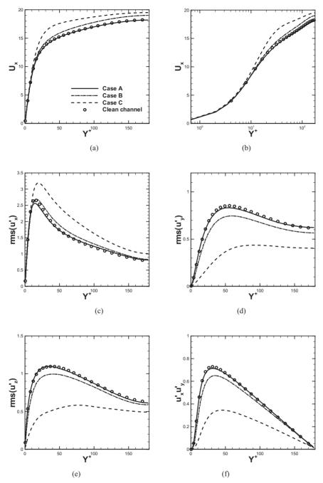
Figure 1 Primary fluid velocity statistics for Case A, B and C. Comparison between particle-free flow (symbols) and particle-laden flows (lines). (a) (b) Mean velocity in the streamwise direction with linear and semi-logarithmic scaling; (c) Velocity fluctuations in streamwise direction; (d) Velocity fluctuations in wall-normal direction; (e) Velocity fluctuations in spanwise direction; (f) Reynolds shear-stress.
