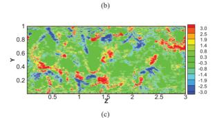
Figure 4. Instantaneous flow contours in a cross-sectional (y, z)-plane at the same time instant as in Figure 3. (a) Wall-normal fluid velocity  $u_y$  (colour-contours); (b) wall-normal particle velocity  $v_y$ ; (c) wall-normal component of the drag force  $-f_y^p$  from the fluid on the particles.
