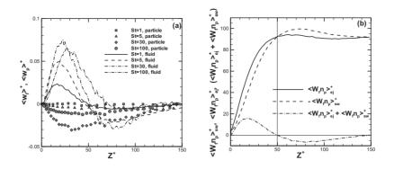
FIG. 1: (a) Mean values of the wall-normal component of the fluid velocity seen,  $\langle w_f \rangle^+$ , and of the particle velocity,  $\langle w_p \rangle^+$ . (b) Density-weighted fluid velocities seen by particles entrained in ejections or sweeps for St=5.
