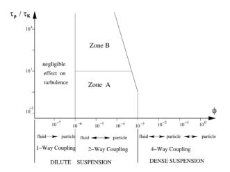
FIGURE 2.4. The map of different coupling regimes based upon volume fraction  $\Phi$  from Elghobashi (2006).  $\tau_p$  is the particle response time and  $\tau_k$  is the Komogorov time-scale.
