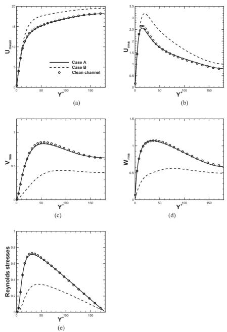
**Figure 1.** Comparison between the unloaden channel flow ( $\circ$ ) and particle-laden flows (— Case A and – – Case B). (a) Mean velocity distribution; (b) Velocity fluctuations in streamwise; (c) Velocity fluctuations in wall-normal; (d) Velocity fluctuations in spanwise; (e) Reynolds shear stress.
