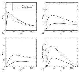
FIG. 2. Turbulence intensities and Reynolds shear stress for the particleladen channel flow (solid lines) and for the unladen flow (broken lines). (a) Streamwise intensity  $u_{\rm rms}$ ; (b) cross-stream intensity  $v_{\rm rms}$ ; (c) wall-normal intensity  $w_{\rm rms}$ ; and (d) Reynolds shear stress  $-\overline{uw}$ .
