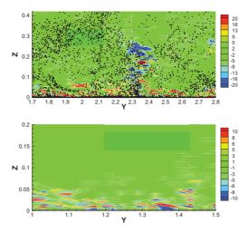
FIGURE 1. Instantaneous feedback in the streamwise direction from the spheroidal particles on the flow field. Near-wall contour plots in the cross-sectional plane of (a)particle-force  $f_x^P$ ; and (b)the torque-force  $\partial T_{jx}^P/\partial x_j$ . The coordinates Y and Z in the spanwise and wall-normal directions, respectively, are scaled with h and Z = 0.1 corresponds to  $z^+ = 36$ .
