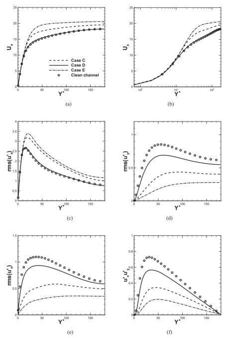
Figure 2 Primary fluid velocity statistics for Case C, D, and E. Comparison between particle-free flow (symbols) and particle-laden flows (lines). (a, b) Mean streamwise velocity in the streamwise direction; (c) Velocity fluctuations in streamwise direction; (d) Velocity fluctuations in wall-normal direction; (e) Velocity fluctuations in spanwise direction; (f) Reynolds shear stress.
