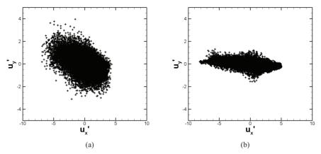
Figure 9. Scatter plot of the instantaneous velocity fluctuations in the wall-normal versus the streamwise direction at  $Y^+ \approx 38$ . (a) Unladen channel flow; (b) particle-laden channel flow.
