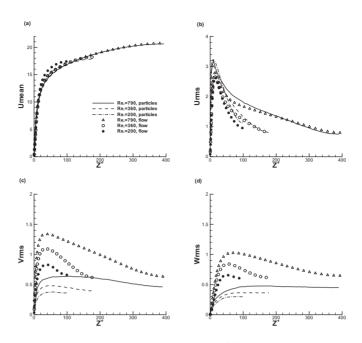
Figure 8: Comparison between fluid and particle mean velocity (a) and velocity fluctuations in the streamwise (b), spanwise (c), and wall-normal (d) directions for  $\tau^+$ =100. The symbols denote fluid velocities and the lines represent particle velocities. The profiles are terminated at the mid-plane of the channel.
