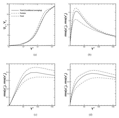
Figure 7. Comparion between tranditionally sampled fluid statistics and conditionally-sampled results on the particle positions. (a) Streamwise mean velocity; (b) streamwise velocity fluctuations; (c) wall-normal velocity fluctuations; (d) spanwise velocity fluctuations.
