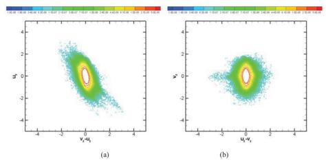
Figure 12. Scatter plot of spanwise velocity components. (a) Fluid velocity versus slip velocity; (b) particle velocity versus slip velocity.
