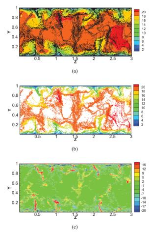
Figure 3. Instantaneous flow contours in a cross-sectional (y, z)-plane. (a) Streamwise fluid velocity  $u_x$  (colour-contours) and point-particle distribution (black dots); (b) streamwise particle velocity  $v_x$ ; (c) streamwise component of the drag force  $-f_x^p$  from the fluid on the particles.
