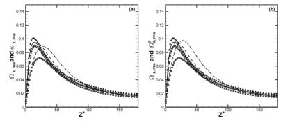
FIG. 6. Comparison between fluid spin intensities  $\Omega_{zrms}$  (symbols), conditionally averaged fluid spin intensities  $\Omega_{zrms}^{P}$ (lines), and particle spin intensities  $\omega_{zrms}$  (lines).  $\tau_{t}^{+} = 1$ : triangle and solid line;  $\tau_{t}^{+} = 5$ : open circle and dashed line;  $\tau_{t}^{+} = 30$ : square and dash dot line. (a) fluid and particles and (b) fluid and conditionally averaged fluid at particle positions.
