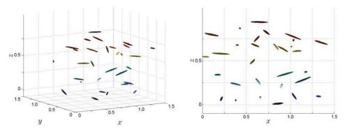
Figure 2: Instantaneous orientation of non-spherical particles in a turbulent channel flow. The orientation of the prolate spheroids varies in time and with position. A perspective view is shown to the left and a planar view to the right. Statistics of the particle orientations are deduced from the instantaneous orientations.
