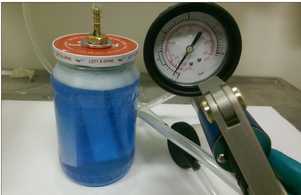
Figure 5-4 Vacuum infusing specimens with RIMR135 epoxy. The vacuum forces air out of the porous paper material, frothing the liquid agent—a good sign.
