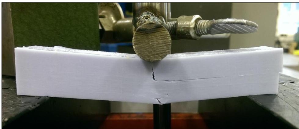
Figure 5-10 Failure along the mid plane of epoxy infused specimen “20–”
