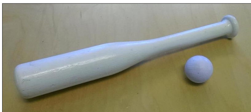
Figure 3-4 Lacquered bat and ball printed with IRIS
