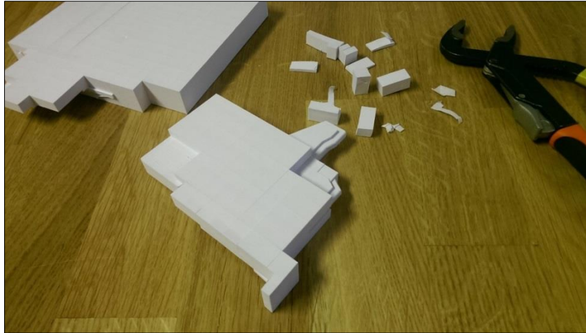
Figure 3-3 De-cubing a part after print
