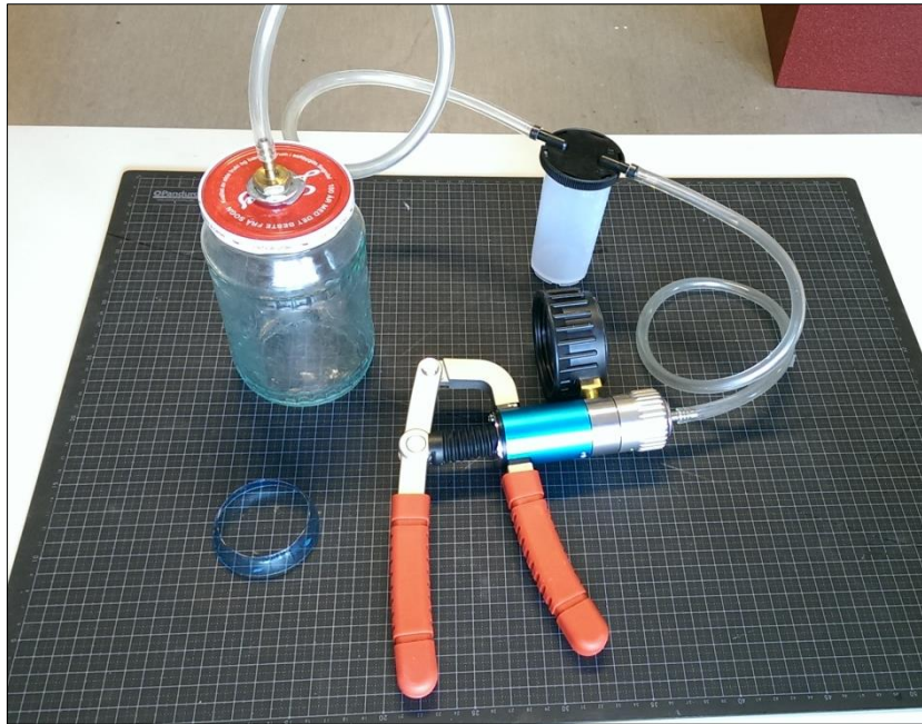
Figure 5-3 Vacuum infusion equipment for quantitative specimens
