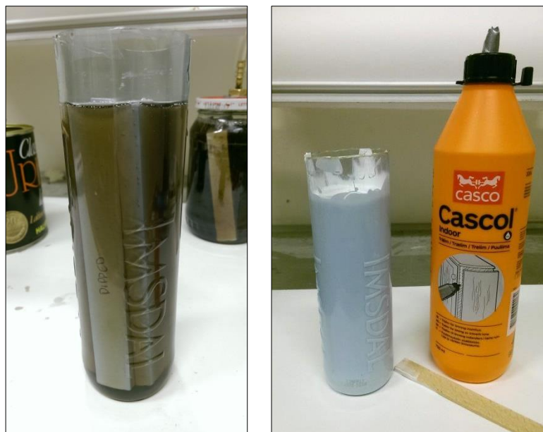
Figure 5-5 Soaking specimens in Classic Uretan Lakk (left) and wood glue (right)
