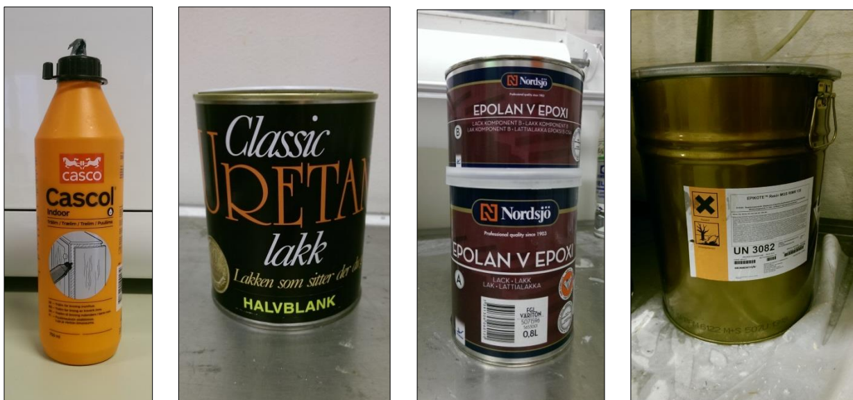
Figure 5-2 Hardening agents explored during the quantitative testing. Form the left: Casco Indoor, Classic Uretan Lakk, Epolan V Epoxi Lakk, RIMR 135 resin.
