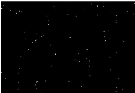
Figure 4.7: P3A01 - 1900: Coarse grained material. 250X magnification. Particle area fraction of 0.12 %.
