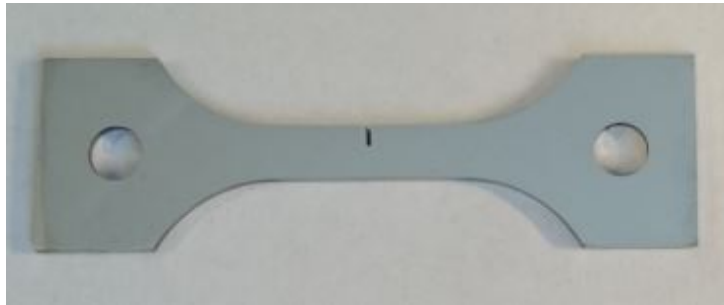
Figure 3.4: Appearance of a sample after grinding and polishing.
