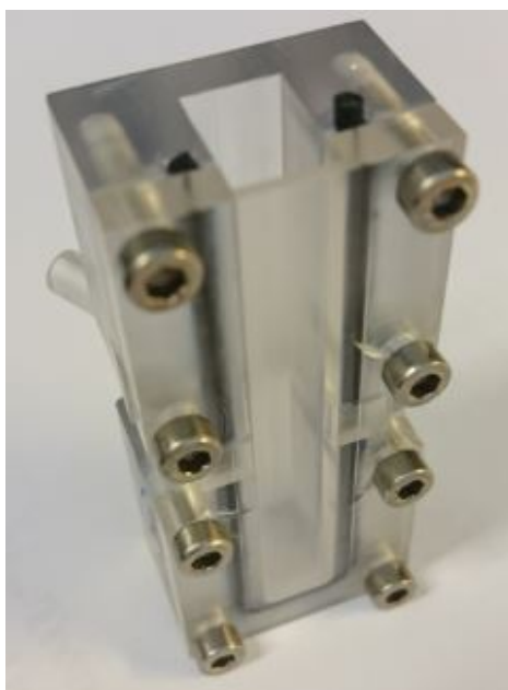
Figure 3.9: The old design for the electrolyte chambers. The front panel is made from polycarbonate, polished to make the sample visible.
