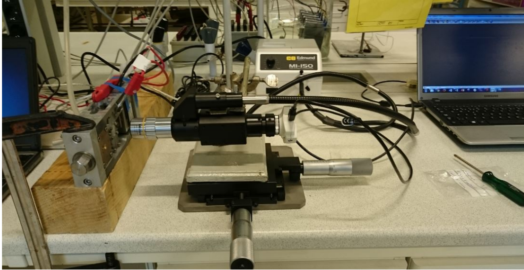
Figure 3.6: Initial setup for the microscope showing the microscope connected to a 10X objective, digital camera, light source and micro movement stage. The digital camera is connected to a computer.
