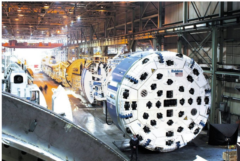
Figure 3.1: The TBM used in Røssåga. Photo provided by The Robbins Company [41].
