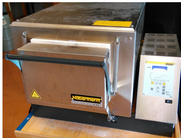
Figure 3.7: The Nabertherm N 17 furnace used for specimen tempering.
