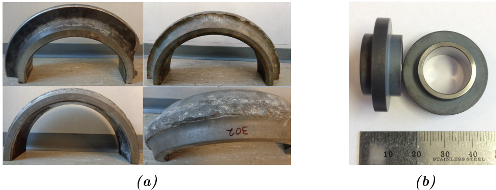
Figure 3.2: a) 19" samples from Røssåga. b) H13 mini-cutters for small scale testing.
