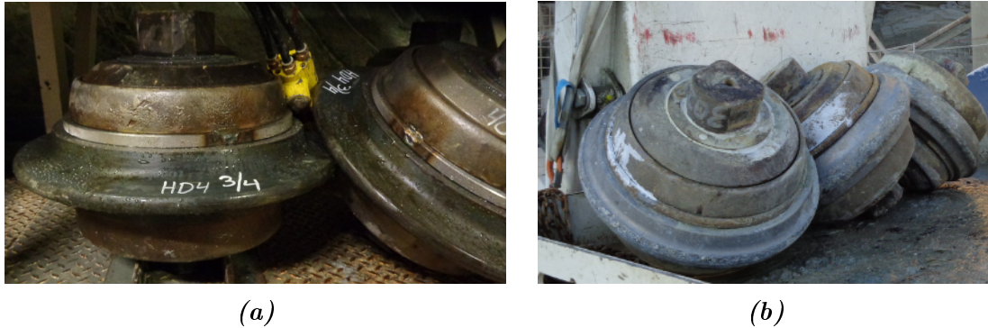
Figure 2.4: a) Cutters with new outer rings ready for use. b) Worn discs replaced due to general wear.
