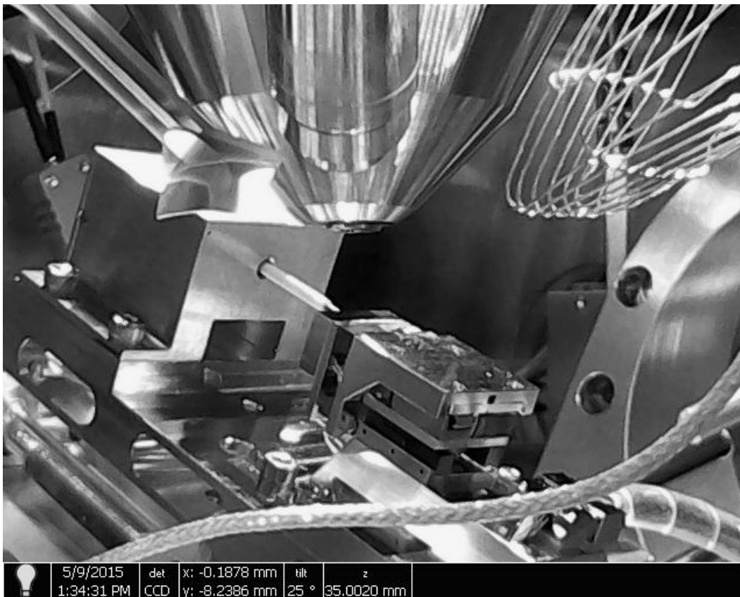
Figure 3.14: The inside of the SEM chamber with the picoindenter installed.
