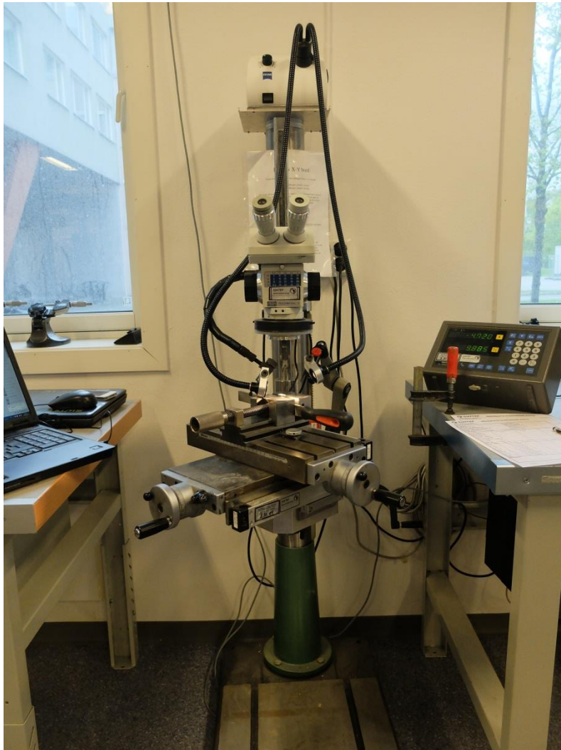
Figure 29 - Technical 2 for crack depth measurement
