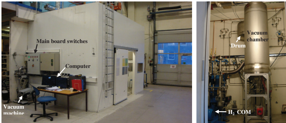
Fig. 3.1 – Complete construction of: (a) the test room, and (b) inside the test room.
