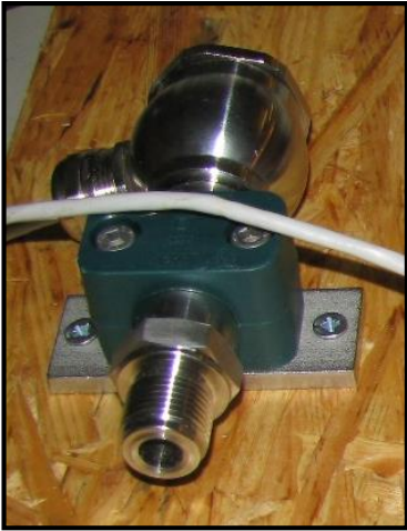
Figure 69: Atmospheric sensor GT402 attached to chipboard
