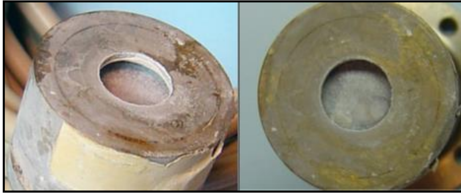
Figure 18: Picture of sensor type 3 with open flush. The element is in the middle and it is covered with a 100 micron thick layer of calcium
