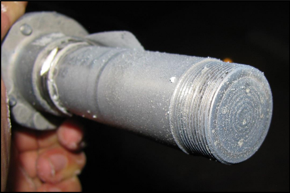
Figure 82: Visual inspection of the new prototype without coating in front and the membrane
