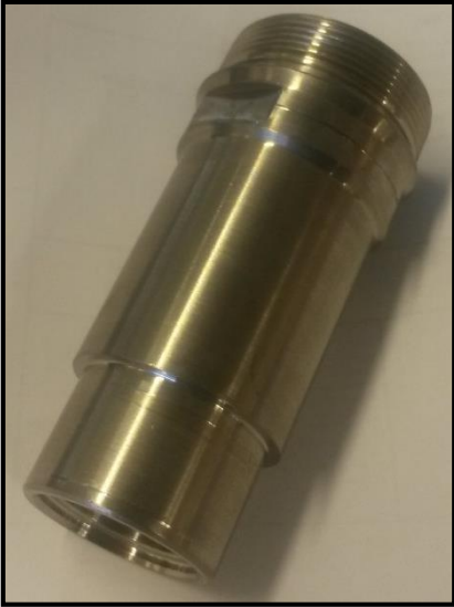
Figure 55: Adjusted housing (removed threads)
