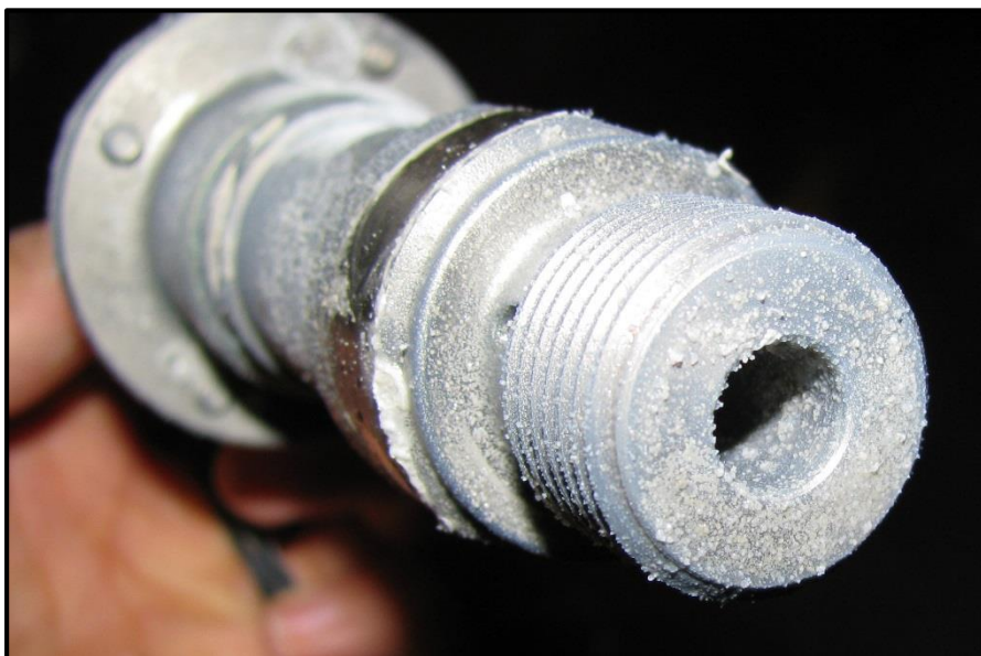
Figure 79: Visual inspection of GT403 in front (process inlet)
