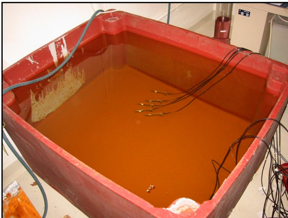
Figure 23: Sensors in tank during earlier Parylene experiment
