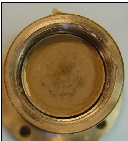
Figure 19: Picture of sensor type 5. As a result of not grounding the sensor via the house, no chemical reactions yield deposition of calcium at the membrane surface
