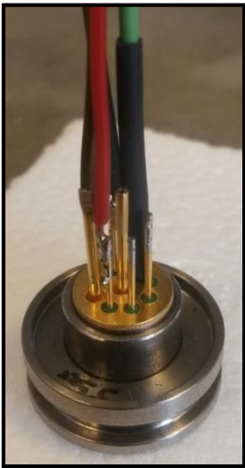
Figure 44: Wires soldered to pins on element
