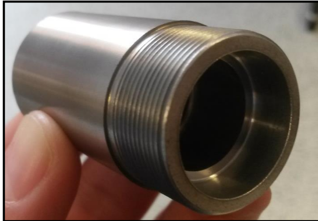
Figure 51: Lowermost housing part with threads
