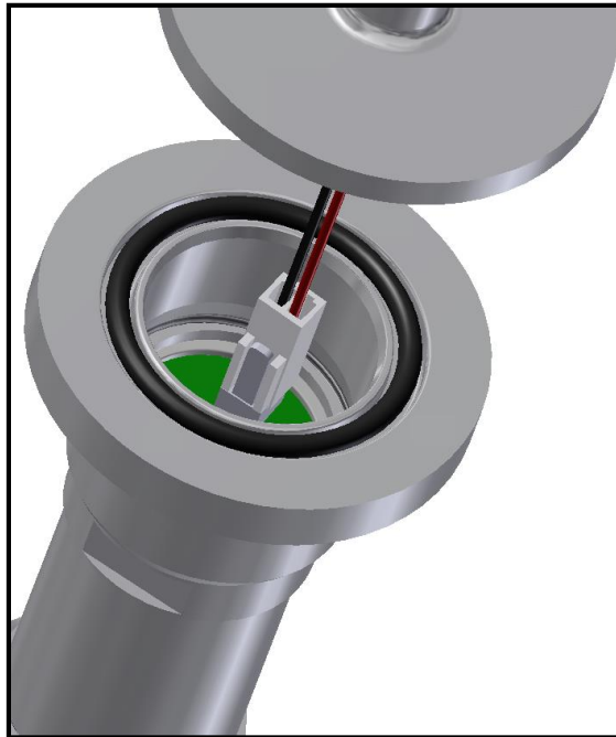
Figure 71: CAD-model: Connecting wires from cable to sensor
