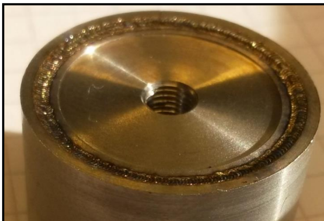
Figure 43: Middle part is below the outer tube
