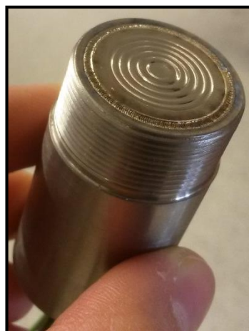
Figure 49: Element laser welded to housing
