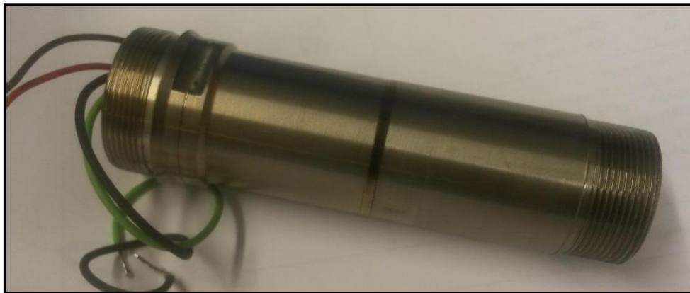
Figure 58: Laser welded housing connection
