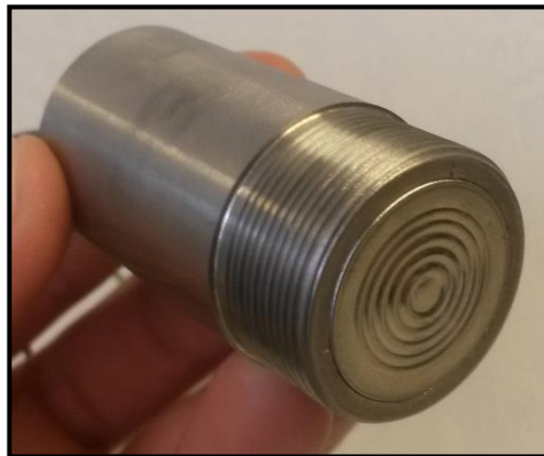
Figure 50: Lowermost housing part and element in flush position
