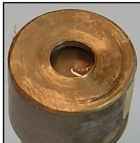
Figure 20: Picture of sensor type 4 with open flush. The silicone gel cover is intact and no calcium layer has been deposited to the membrane
