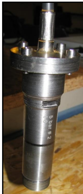
Figure 72: New generation pressure transmitter ready for submersion
