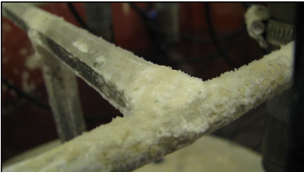
Figure 78: Thick deposition layer on welds at the sensor attachment creation
