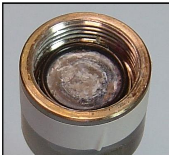
Figure 17: Picture of type 1. A 100 micron thick layer of calcium has deposited to the membrane surface of the pressure element
