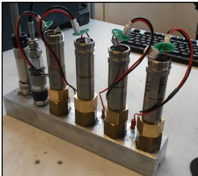
Figure 60: Pressure testing after assembling housing and PCB
