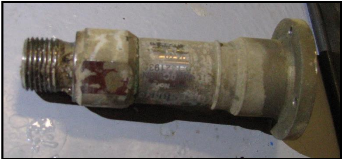
Figure 30: Another defect Sensor on KV Bergen
