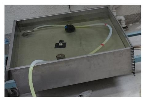
*Figure (3. 7): Tank used for DWH riser experiments (0.95 x 0.95 x 0.4 meters)*
