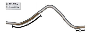
Figure (5. 1): Main oil slug accumulating in upstream section of buoyant loop [4]
