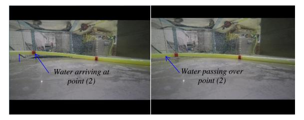
*Figure (5. 14): Left image shows slug filling until point (2), right image shows slug passed point (2) pushing the buoyant loop to a lower depth*
