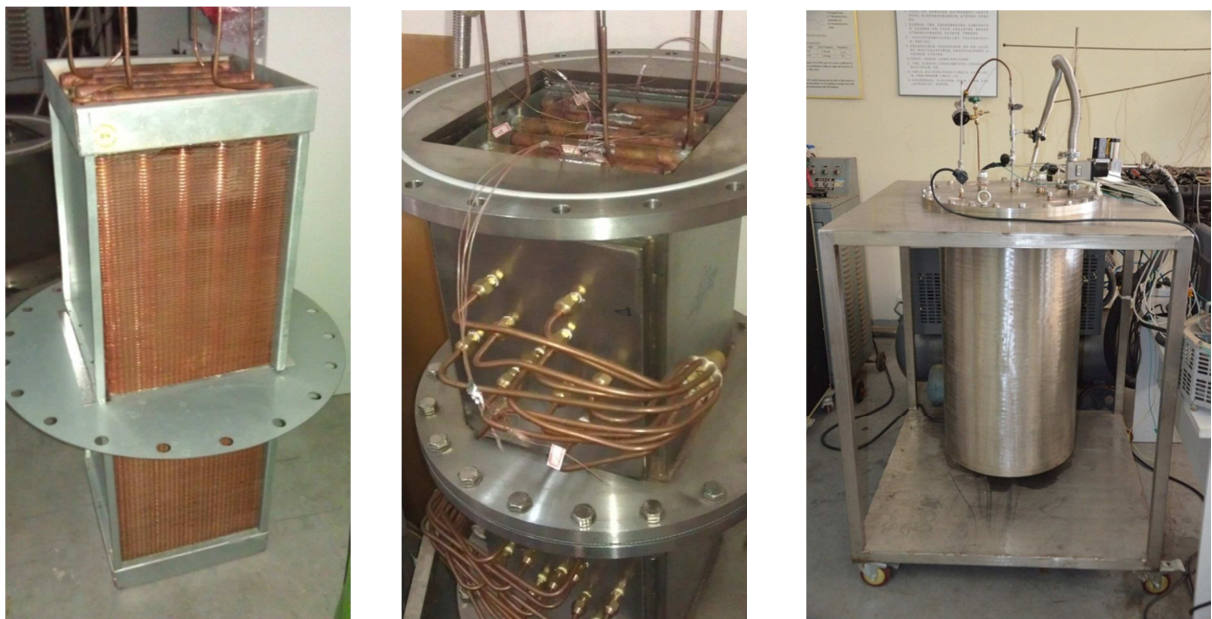
Figure 5-4 heat pipe heat exchanger (from left to right: heat pipes and vertical distribution plates, distribution caps, heat exchanger in vacuum hull)
