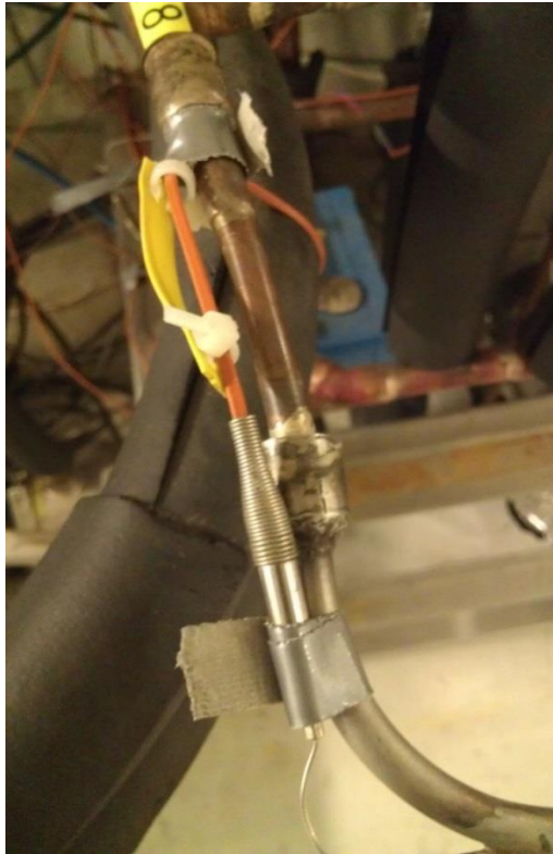
Figure 7 Thermal couple in the expander loop
