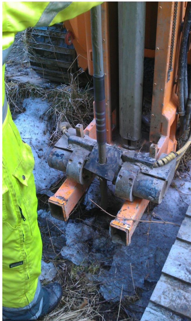
Figure 4.6 Dismantling a rod from the resistivity module after sounding, photo by S.P.
