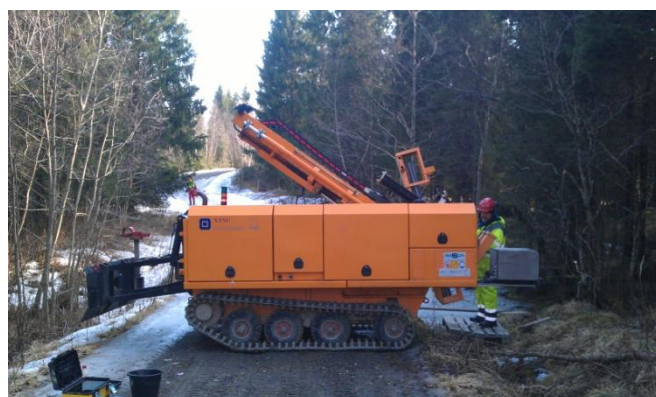
Figure 4.5 Heavy geo-rig, photo by S.P.
