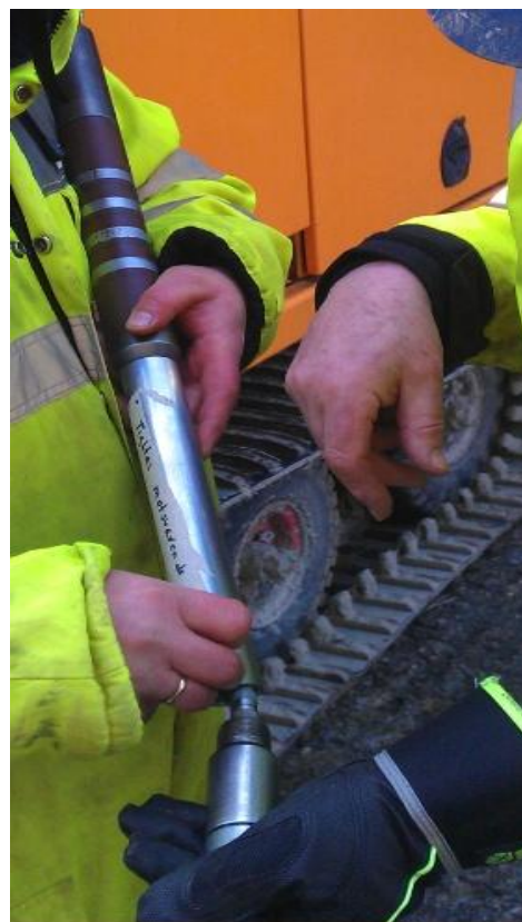
Figure 1.2 Connected resistivity module to piezocone, photographed by S.P.
