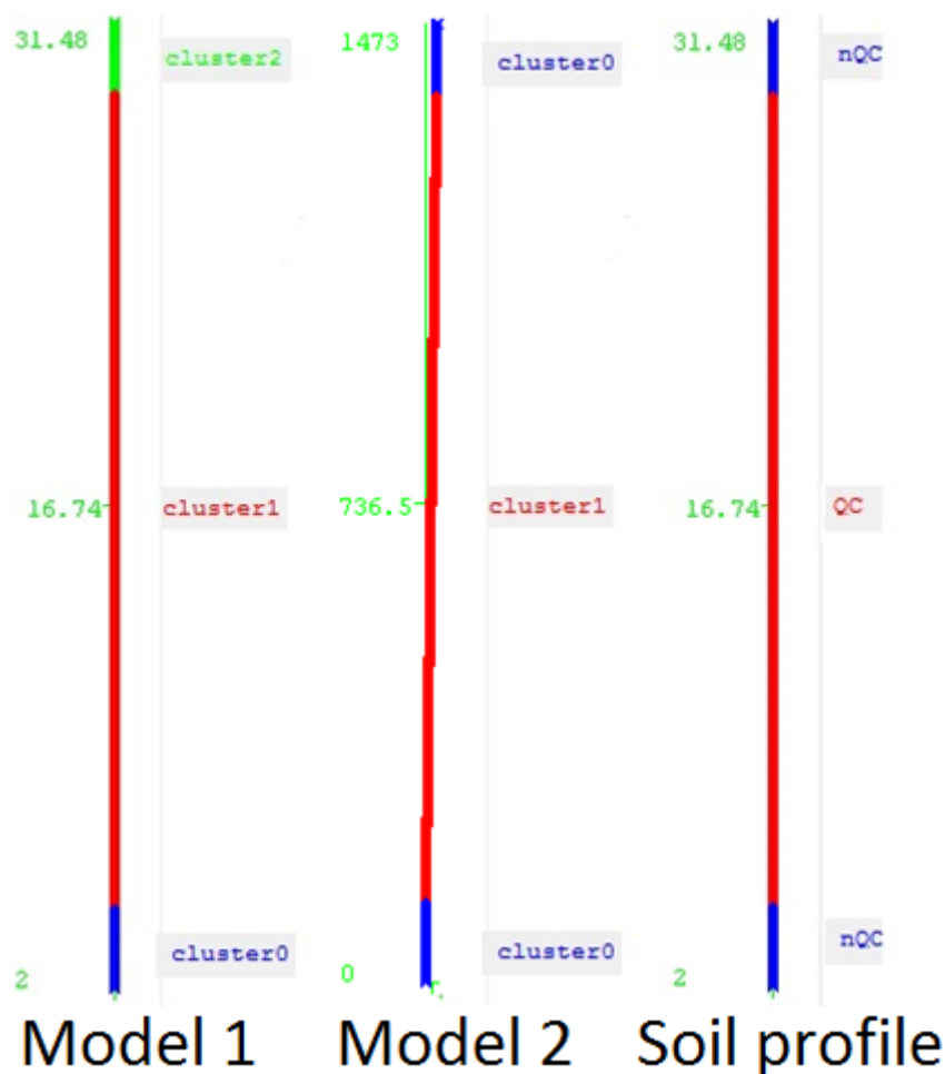
Figure 7.11 Cluster assignments in trained models 1) & 2) compared with soil class attribute 3) in Fallan BP 2
