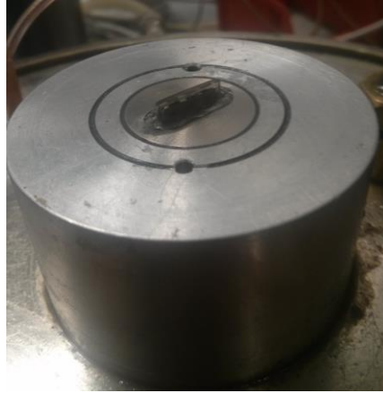
Figure 4.14 Piezoelectric bender element fitted into modified pedestal (Photo: Eide, H)
