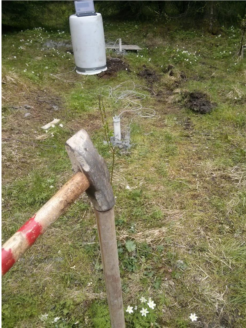
Figure 4.7 Setup of the crosshole test at Tiller (Photo: Eide, H)
