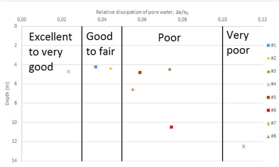
Figure 6.8 Measure of sample quality based on relative dissipation of pore waver
