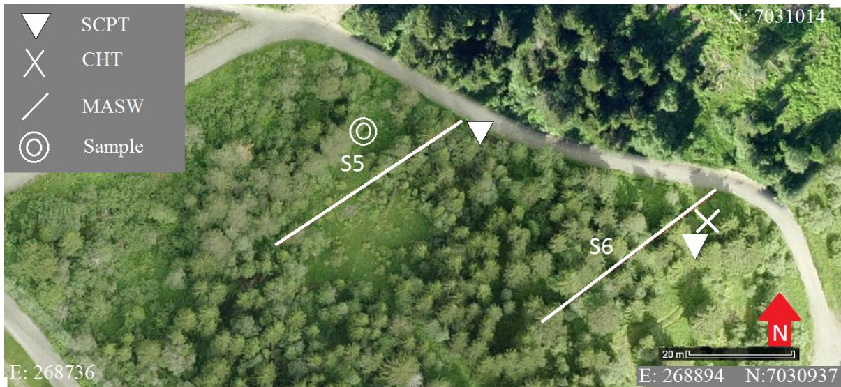
Figure 3.3 Overview of Tiller and approximate locations of performed site investigations
